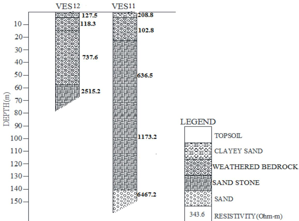
Figure 2: Geoelectric Sections of the 1D Sounding
