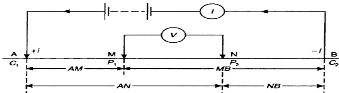
Figure 1: Generalised form of electrode configuration in resistivity surveys
