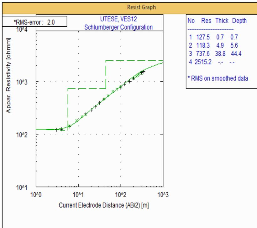
Figure 3: VES Curves for 1D Sounding
