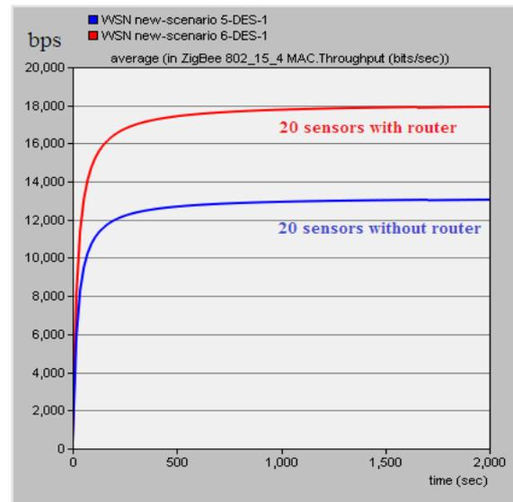
Figure 11 Throughput with and without a router for 4 coordinators
