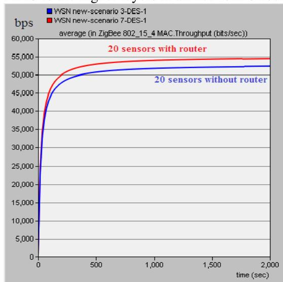
Figure 10 Throughput with and without a router for a single coordinator
