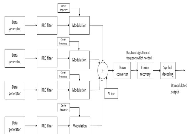
Fig.1 Block diagram of multicarrier demodulator
