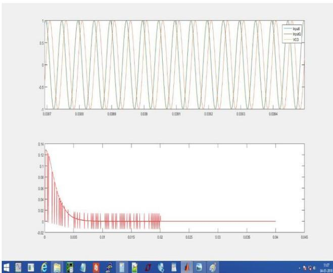
Fig. 5 costas loop simulation in MATLAB
