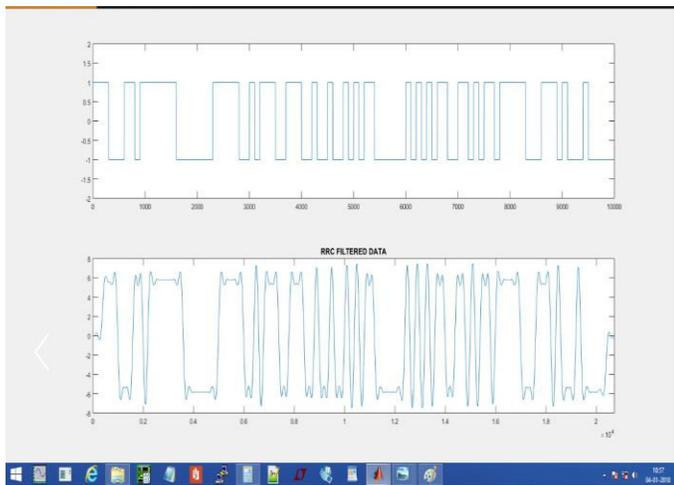
Fig.2 Pulse shaping of data using rrc filter
