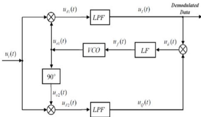
Fig. 4 costas loop block diagram
