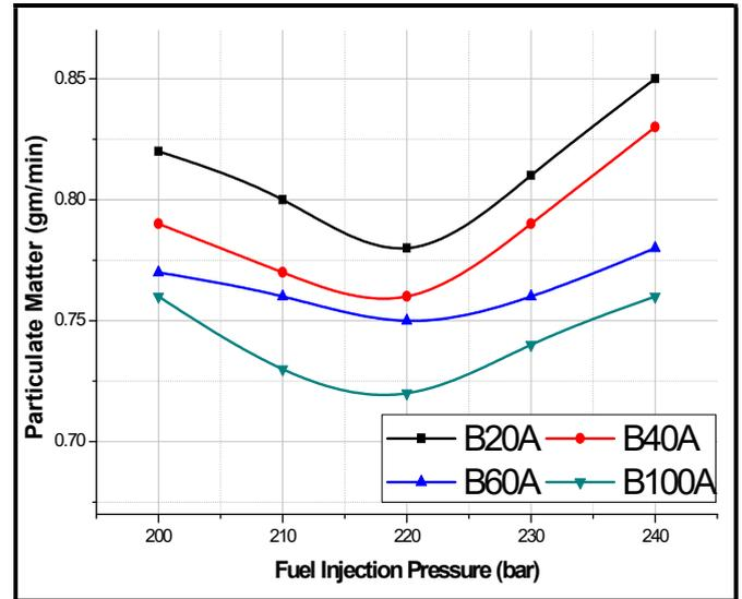
Fig. 6: Variation of Emission of Particulate Matter with Different Fuel Injection Pressures for tested blends
