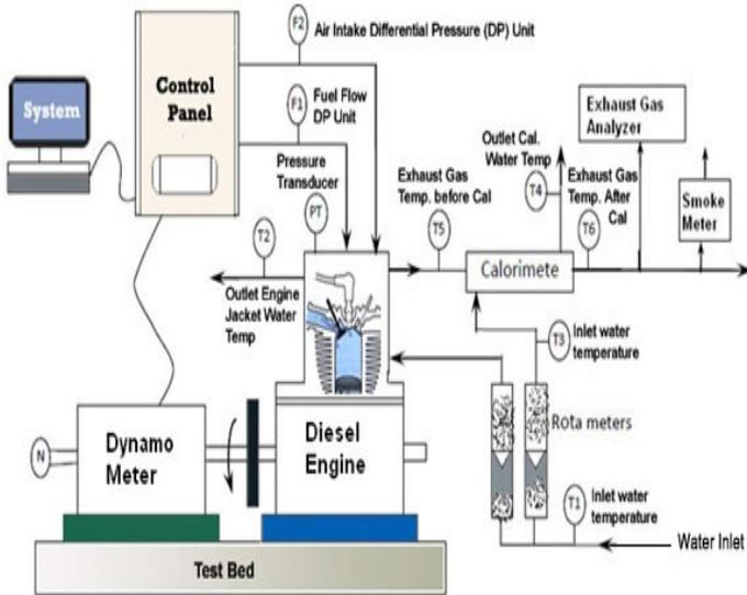
Fig. 2: Schematic Diagram of Experimental Setup
