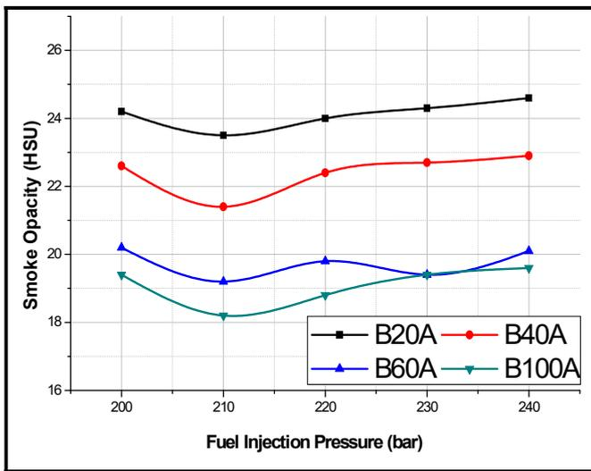
Fig. 5: Variation of Emission of Smoke Opacity with Different Fuel Injection Pressures for tested blends
