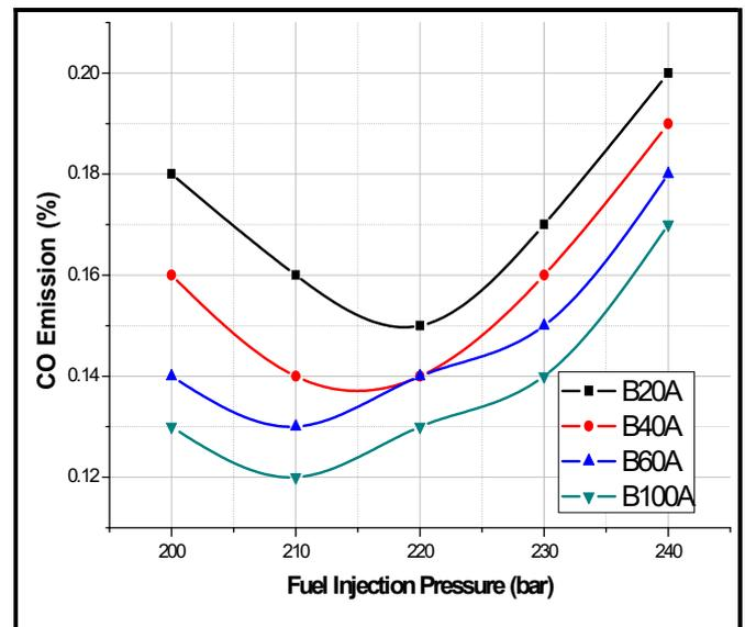
Fig. 4: Variation of CO Emission with different Fuel Injection Pressures for tested blends
