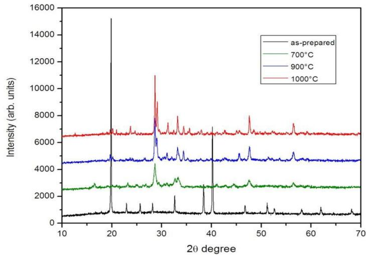
**Fig.1. XRD patterns of  $\text{Sr}_3\text{Gd}_{1.86}\text{Tb}_{0.14}(\text{BO}_3)_4$  powders calcined at various temperatures.**
