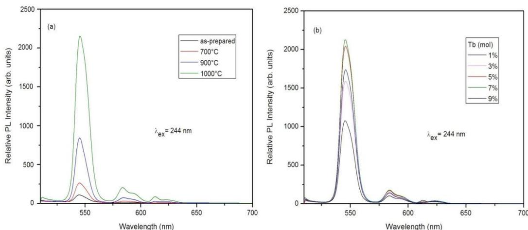
**Fig.4. (a) Emission spectra of  $\text{Sr}_3\text{Gd}_{1.86}\text{Tb}_{0.14}(\text{BO}_3)_4$  showing relative PL intensity as a function of temperature and (b) Emission spectra of  $\text{Sr}_3\text{Gd}_{2(1-x)}(\text{BO}_3)_4:2x\text{Tb}^{3+}$  ( $x=0.01, 0.03, 0.05, 0.07$  and  $0.09$ ) showing variation of emission intensity as a function of  $\text{Tb}^{3+}$  concentrations,  $\lambda_{\text{ex}}=244$  nm.**
