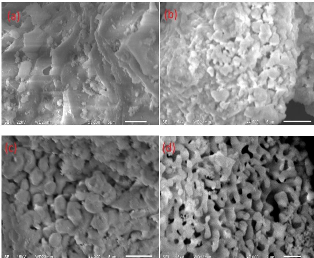
**Fig.2. SEM micrographs of  $\text{Sr}_3\text{Gd}_{1.86}\text{Tb}_{0.14}(\text{BO}_3)_4$  (a) as-synthesized; calcined at (b) 700°C (c) 900°C and (d) 1000°C temperatures.**
