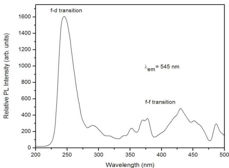
**Fig.3. Excitation spectrum of  $\text{Sr}_3\text{Gd}_{1.86}\text{Tb}_{0.14}(\text{BO}_3)_4$  sample calcined at  $1000^\circ\text{C}$ ,  $\lambda_{\text{em}} = 545$  nm.**
