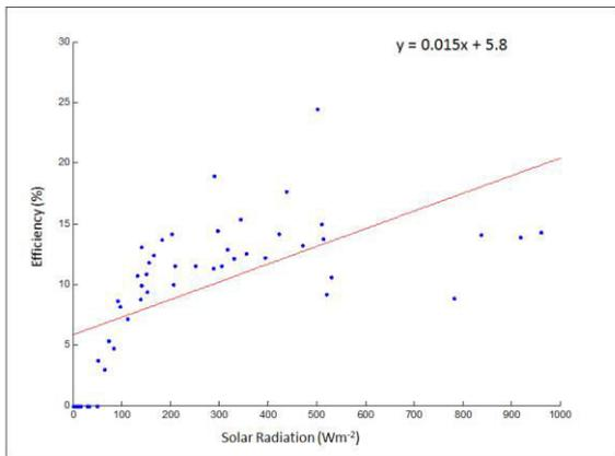
Figure 1 Graph of Monocrystalline Efficiency against Solar Radiation in Calabar
