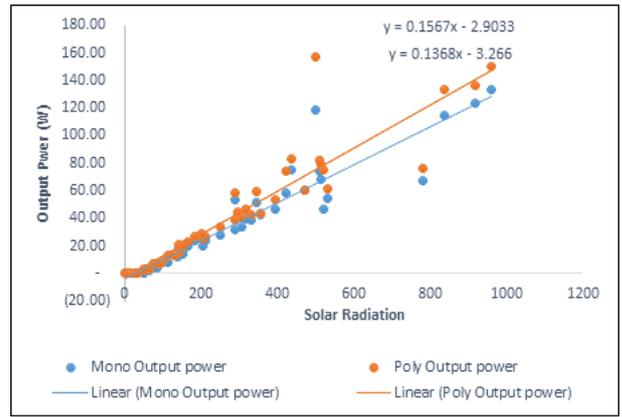
Figure 10 Graph of Output Power against Solar Radiation in Calabar
