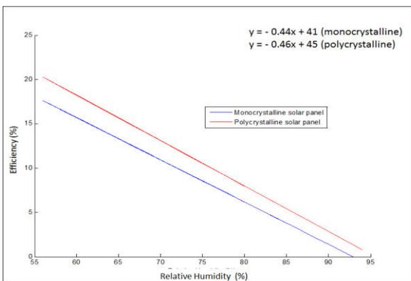
Figure 9 Graph of Efficiency against Relative Humidity in Calabar
