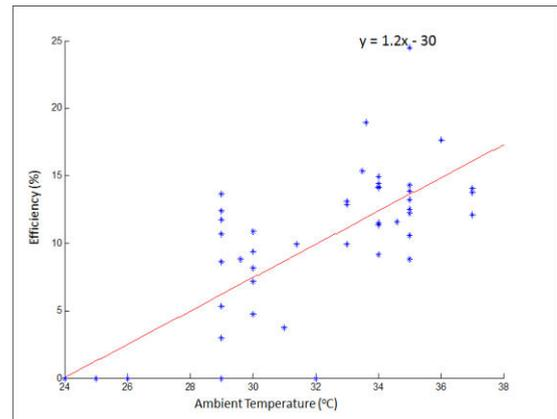
Figure 3 Graph of Monocrystalline Efficiency against Ambient Temperature in Calabar
