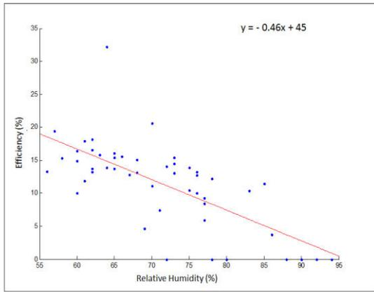
Figure 6 Graph of Polycrystalline Efficiency against Relative Humidity in Calabar
