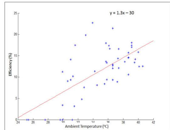
Figure 4 Graph of Polycrystalline Efficiency against Ambient Temperature in Calabar
