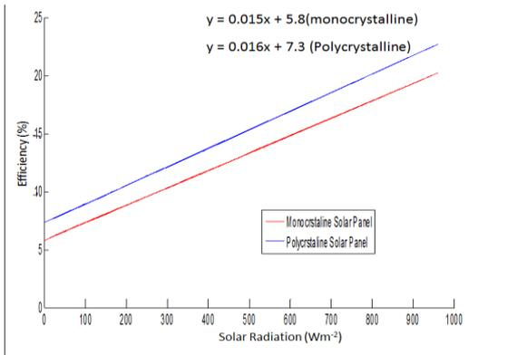
Figure 7 Graph of Efficiency against Solar Radiation in Calabar
