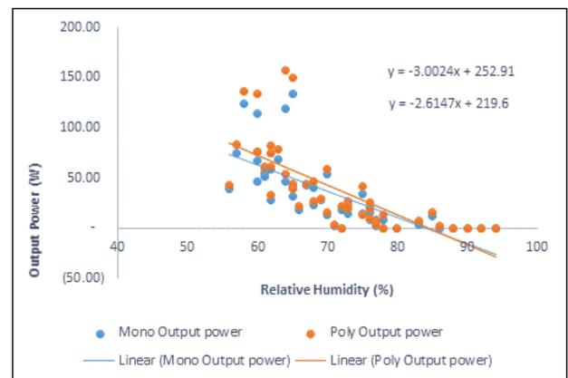
Figure 12 Graph of Output Power against Relative Humidity in Calabar
