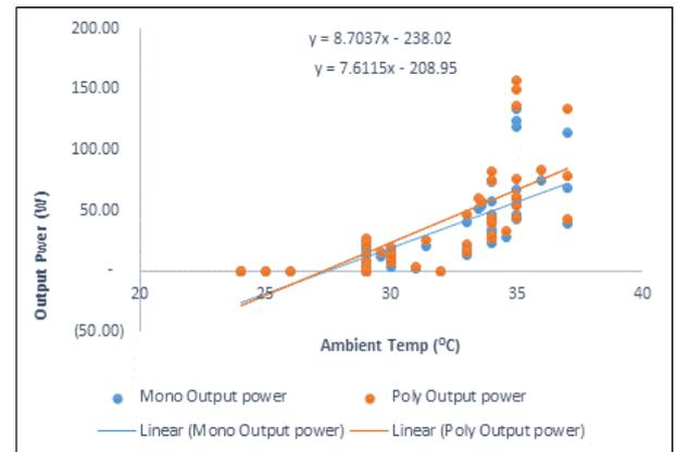
Figure 11 Graph of Output Power against Ambient Temperature in Calabar
