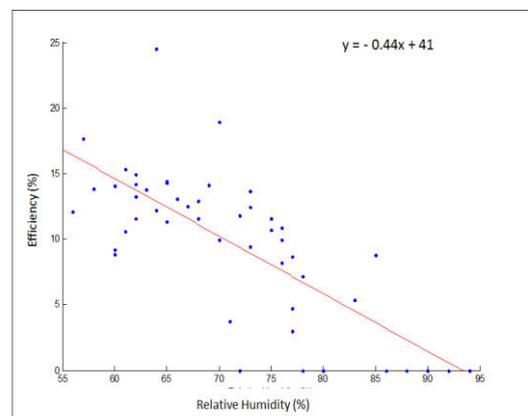
Figure 5 Graph of Monocrystalline Efficiency against Relative Humidity in Calabar
