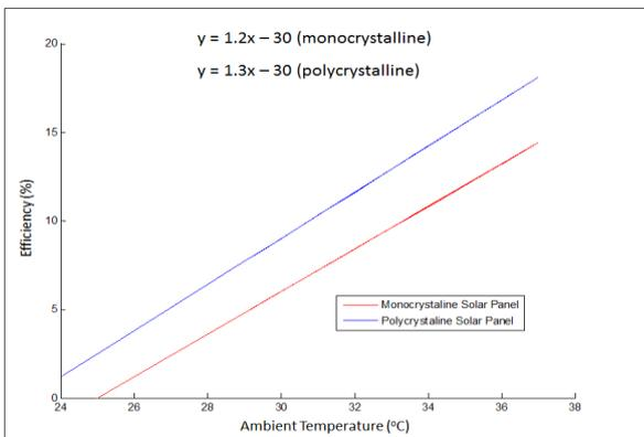
Figure 8 Graph of Efficiency against Ambient Temperature in Calabar
