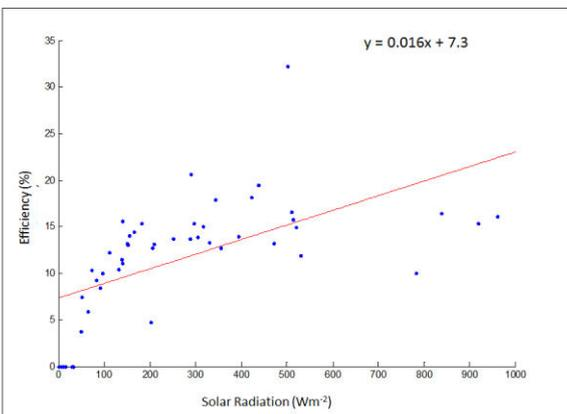
Figure 2 Graph of Polycrystalline Efficiency against Solar Radiation in Calabar
