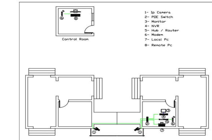
**Figure1. Location of cameras at Electronic gate**
