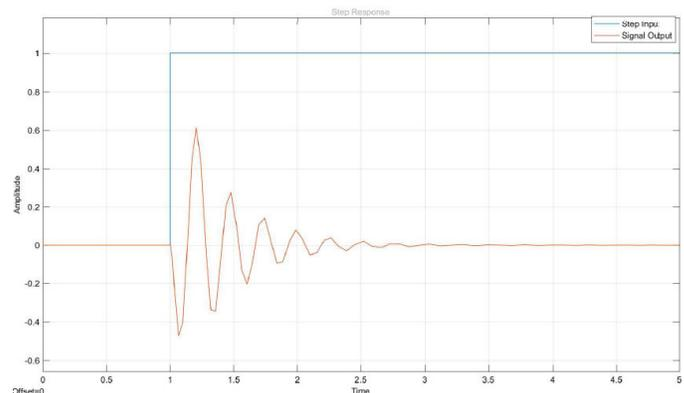
Figure 13: Step Response of a Pneumatic Integrated Suspension System
