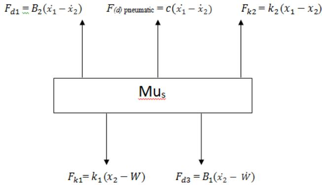
$$\sum F_{ms} = F_{d1} + F_{(d) \text{ pneumatic}} + F_{k2} - F_{k1} - F_{d3} = M_s \ddot{x}_2$$
