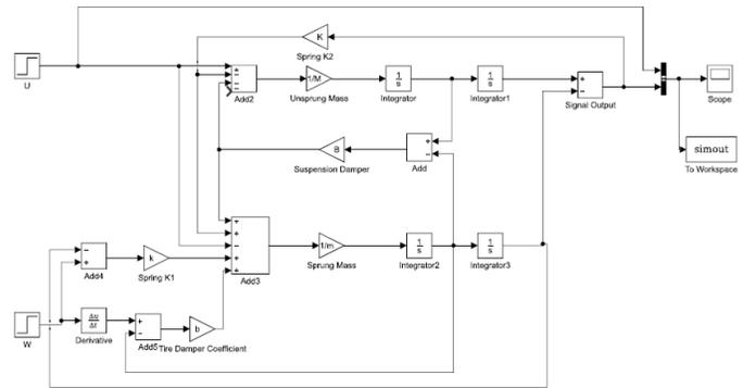
Figure 10: Discrete Block Functions of Matlab Simulink Block Diagram based on conventional passive suspension system
