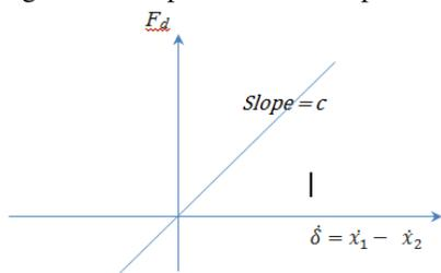
Figure 4: Force versus Separation Velocity
