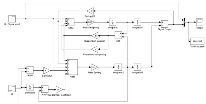
Figure 11: Discrete Block Functions of Matlab Simulink Block Diagram based on new configuration suspension integrated with pneumatic system
