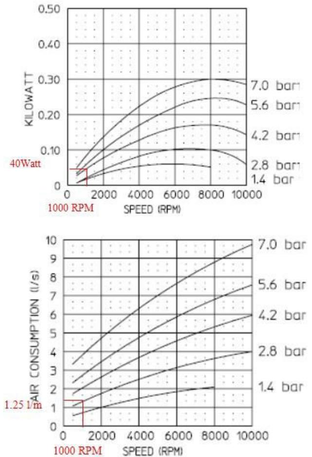
Figure 15: Air Consumption and Power of Air Motor
