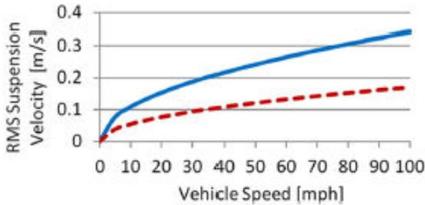
Figure 9 : Velocity analysis over vehicles speeds on good road and average road (solid) [10]
