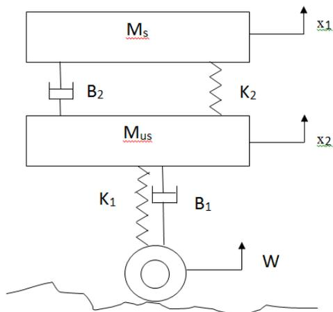
Figure 6 : Passive Suspension of two degree of freedom
