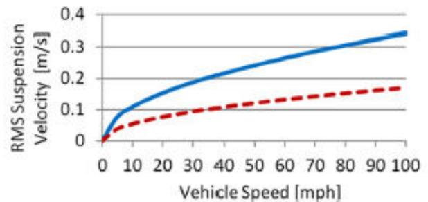
Figure8: Displacement analysis over vehicle speeds; on good road (dashed) and average road (solid) <sup>[10]</sup>
