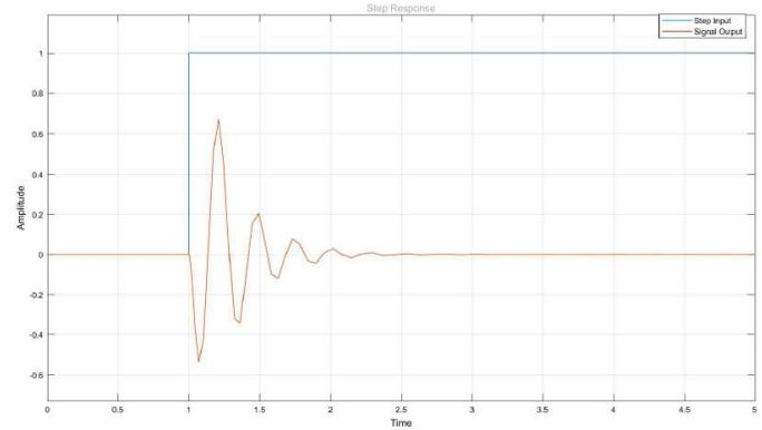
• Figure 12: Step Response of a Normal Passive Suspension System
