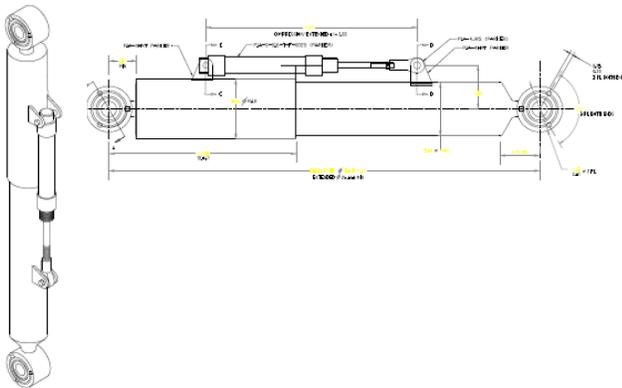
Figure 1: Conceptual design of pneumatic cylinder harvesting energy suspension
