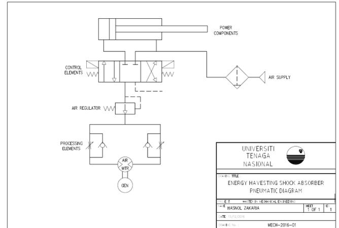
Figure 2: Pneumatic circuit diagram of pneumatic cylinder
