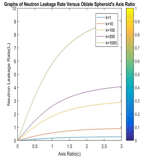
**Fig2:Neutron leakage rate versus axis ratio of aOblatespheroid at various values of k**
