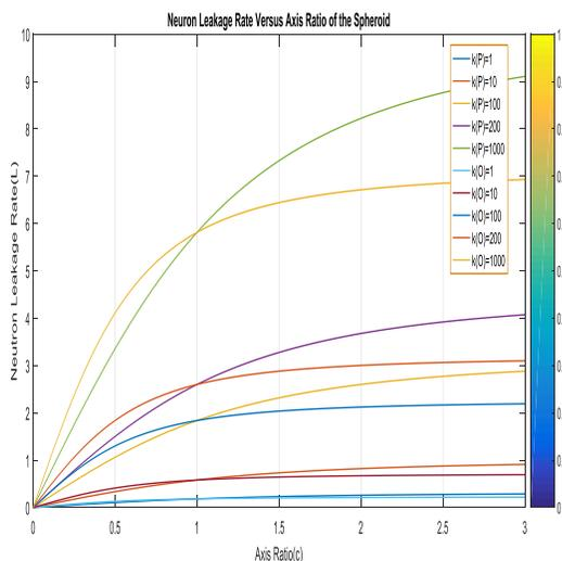
**Fig 4: Neutron Leakage rate versus the Axis Ratio of the Spheroid at various values of  $k$**
