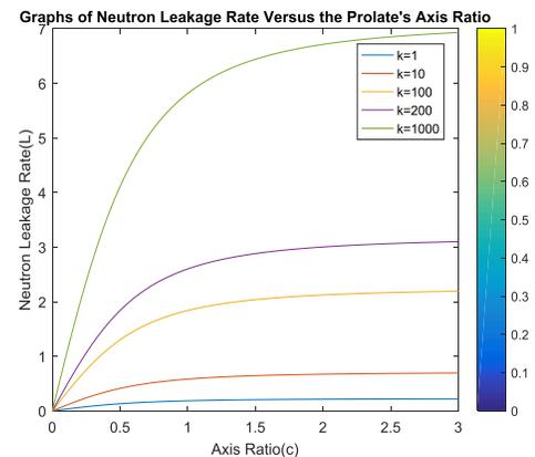
**Fig 3: Neutron leakage rate versus axis ratio of aProlatespheroid at various values of k**
