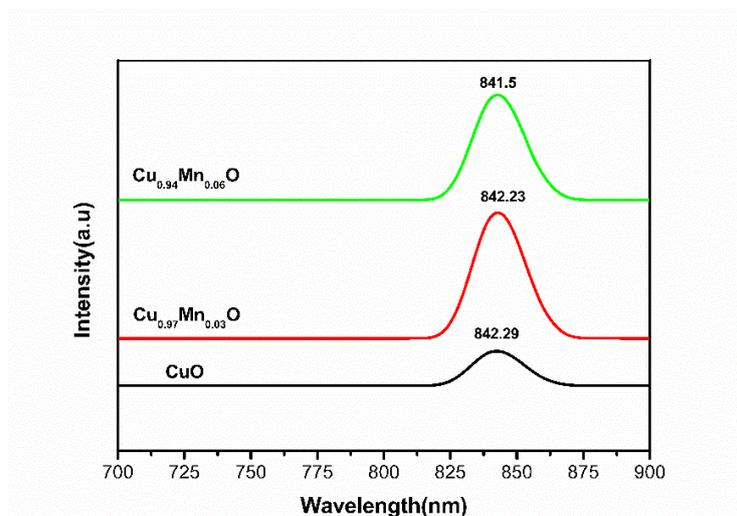
Figure 10. PL spectra of CuO,  $\text{Cu}_{0.97}\text{Mn}_{0.03}\text{O}$  and  $\text{Cu}_{0.94}\text{Mn}_{0.06}\text{O}$  nanoparticles
