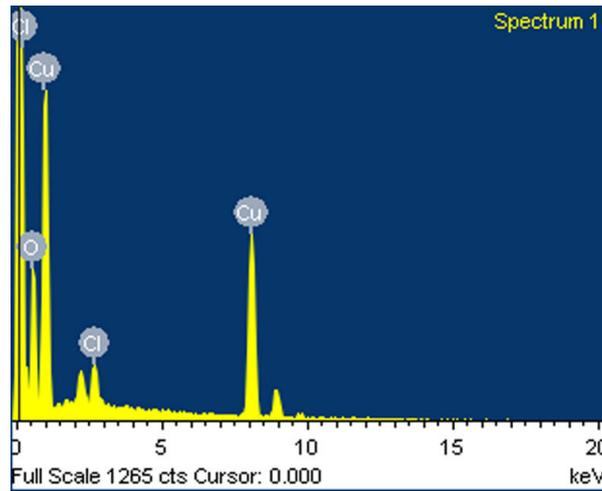
Figure 8. EDAX spectrum of CuO nanoparticles
