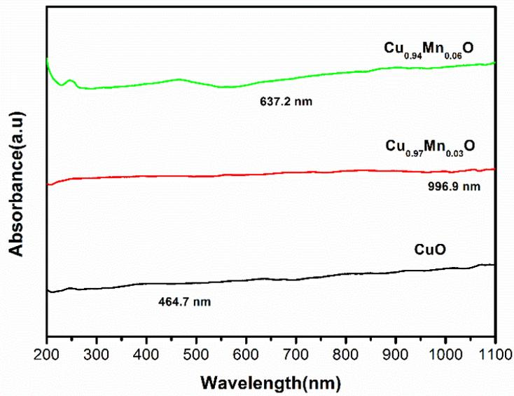
**Figure 2. UV - Visible absorption spectra of the synthesized  $\text{CuO}$ ,  $\text{Cu}_{0.97}\text{Mn}_{0.03}\text{O}$  and  $\text{Cu}_{0.94}\text{Mn}_{0.06}\text{O}$  nanoparticles**
