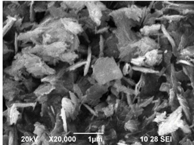
**Figure 5. SEM image of CuO nanoparticles**
