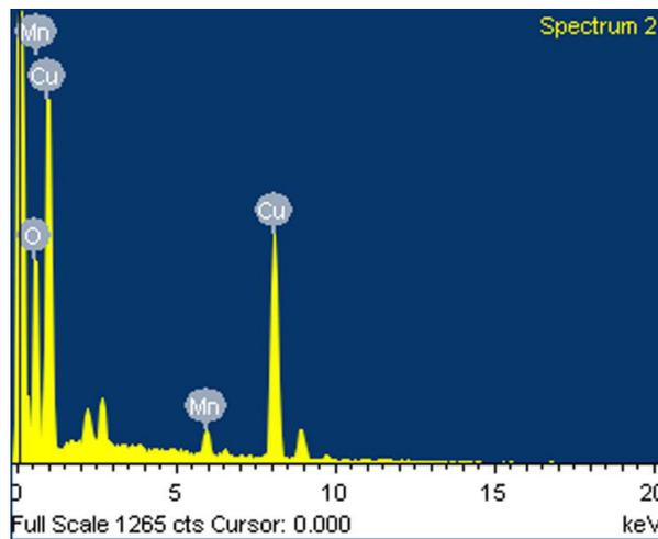
Figure 9. EDAX spectrum of  $\text{Cu}_{0.94}\text{Mn}_{0.06}\text{O}$  nanoparticles
