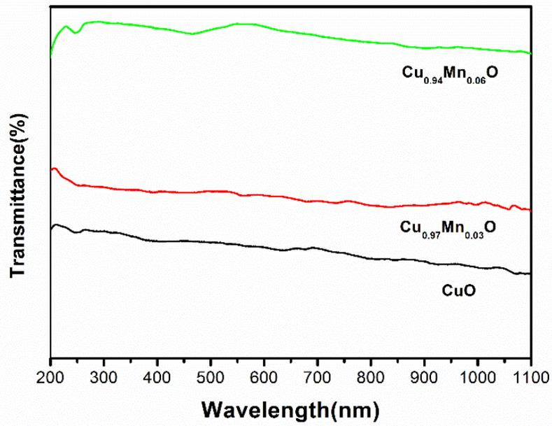
Figure 3 Transmittance spectra of the synthesized CuO, Cu<sub>0.97</sub>Mn<sub>0.03</sub>O and Cu<sub>0.94</sub>Mn<sub>0.06</sub>O nanoparticles
