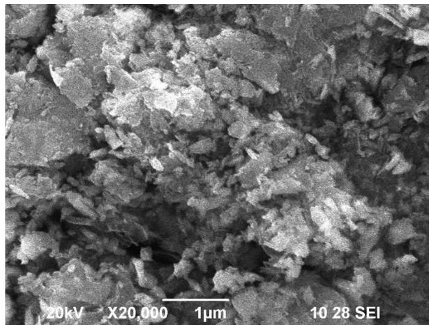
**Figure 6. SEM image of Cu<sub>0.97</sub>Mn<sub>0.03</sub>O nanoparticles**
