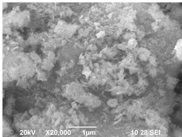
**Figure 7. SEM image of Cu<sub>0.94</sub>Mn<sub>0.06</sub>O nanoparticles**
