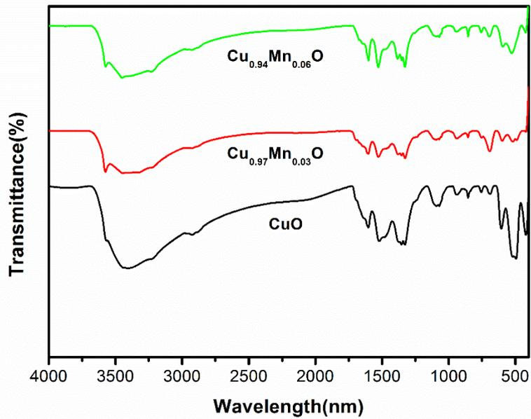
Figure 4 FTIR spectra of CuO, Cu<sub>0.97</sub>Mn<sub>0.03</sub>O and Cu<sub>0.94</sub>Mn<sub>0.06</sub>O nanoparticles
