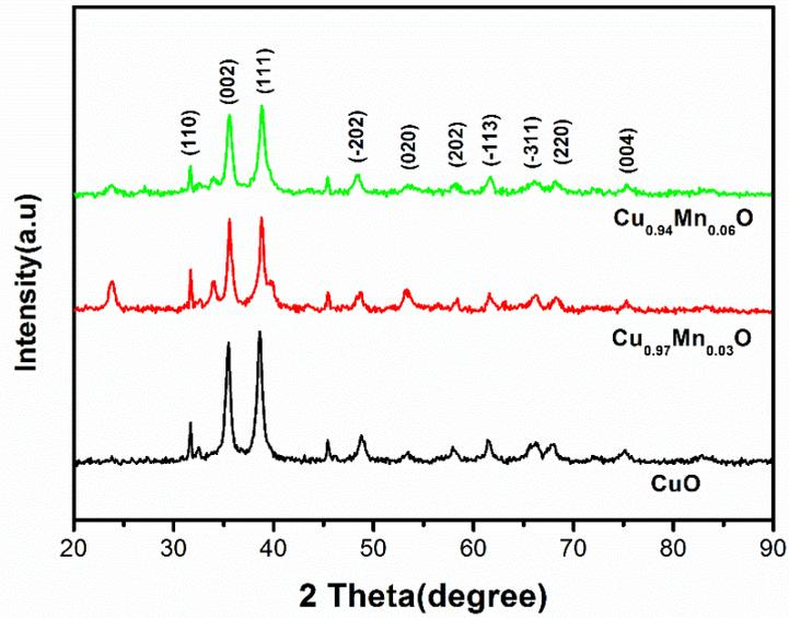
**Figure 1. XRD patterns of  $\text{CuO}$ ,  $\text{Cu}_{0.97}\text{Mn}_{0.03}\text{O}$  and  $\text{Cu}_{0.94}\text{Mn}_{0.06}\text{O}$  nanoparticles**
