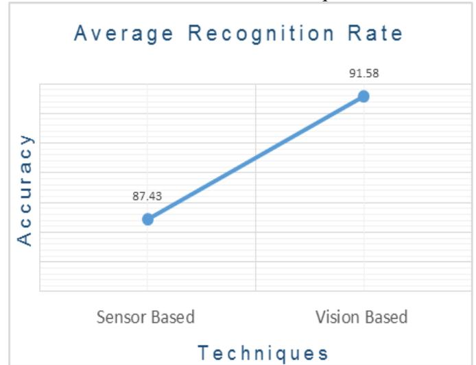
Fig 9. Average Recognition Rate of Sensor Based and Vision Based ASLR Techniques
