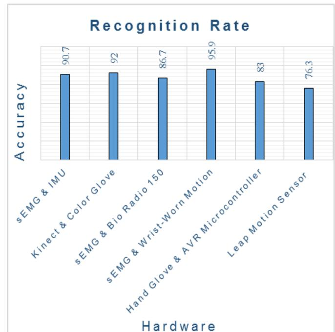
Fig 6. Recognition Rate of Various Sensor Based ASLR Techniques
