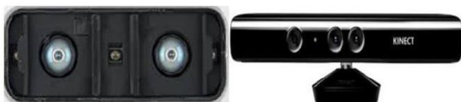
Fig 4. (a) Leap Motion Sensor, (b) Kinect for Xbx360
