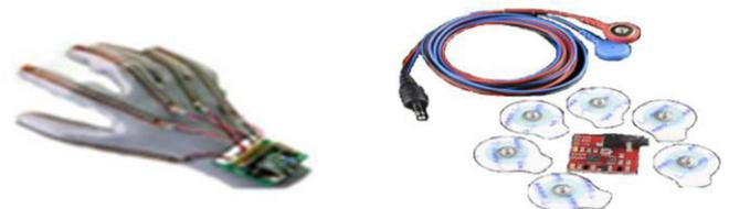
Fig 5. (a) Data Glove with Flex Sensor, (b) sEMG Sensor with cables
