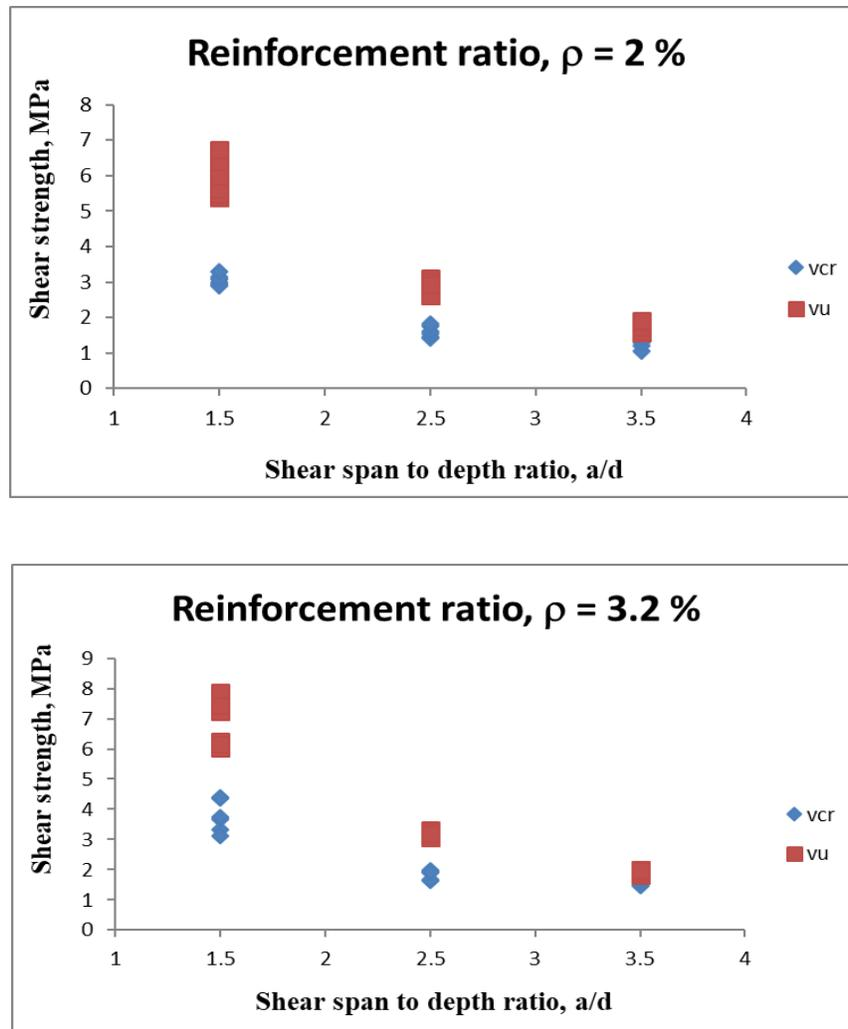
**Fig. 2: Effect of shear span to depth ratio on  $v_{cr}$  and  $v_u$  of RAC beams**
