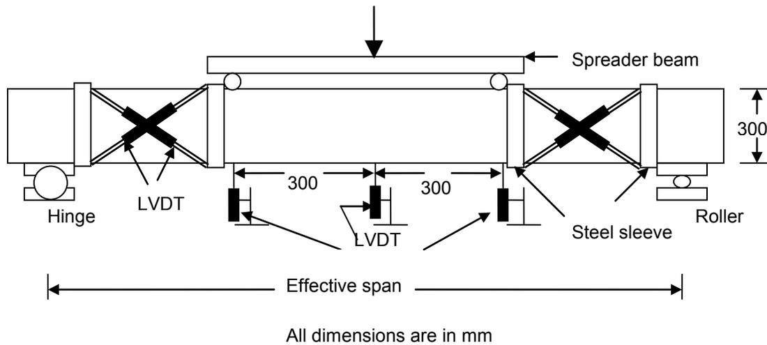
Fig. 1: Test setup configuration for the shear tests
