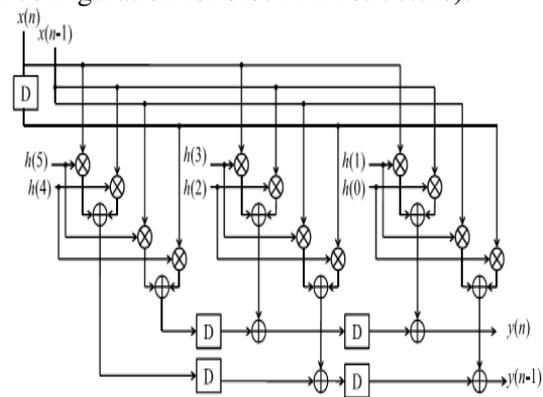
Fig. 2. DFG-4 (retimed DFG-3) transpose form type-II configuration for block FIR structure.
