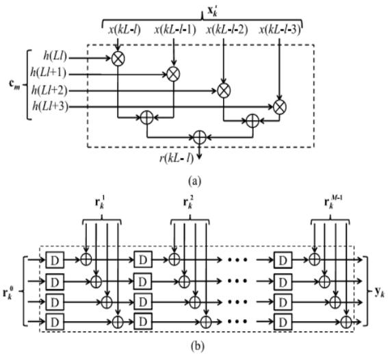
Fig. 5. (a) Internal structure of  $(l + 1)$ th IPC for  $L = 4$ . (b) Structure of PAU for block size  $L = 4$ .
