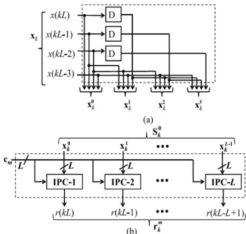
Fig. 4. (a) Internal structure of RU for block size  $L = 4$ . (b) Structure of  $(m + 1)$ th IPU.
