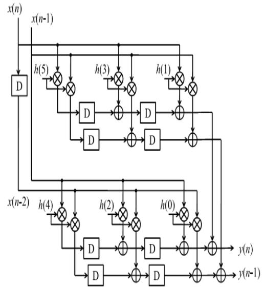
Fig. 1. Merged DFG (DFG-3: transposed from a type-I configuration for block FIR structure).
