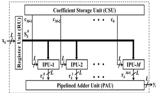
Fig. 3. The proposed structure for block FIR filter.
