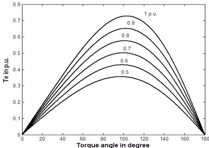
Figure.2 Air gap torque versus torque angle for various stator currents
