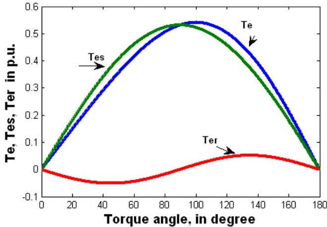
Figure.1 Reluctance, synchronous and air gap torques versus torque angle for stator current magnitude of 1.3 p.u.
