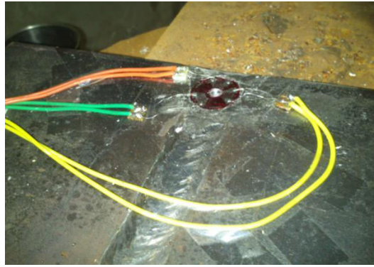
Figure 3.1. Attachment of strain gauges to welded work piece
