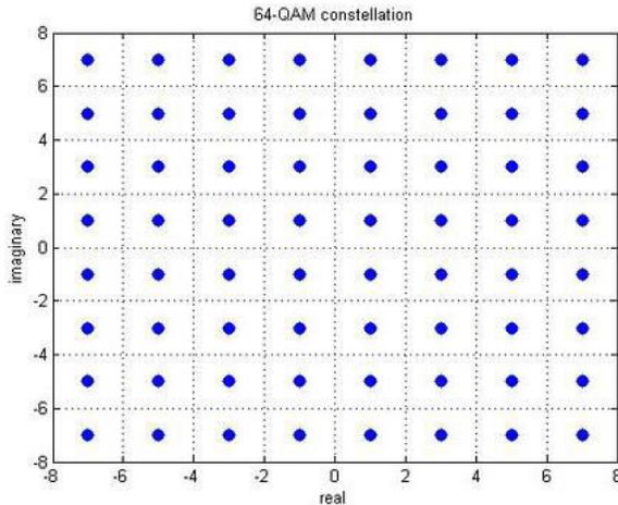
Figure 4 (b) constellation diagram of the produced 64-QAM signal
