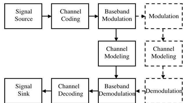
Figure 1, Basic digital-to-analog transmission scheme
