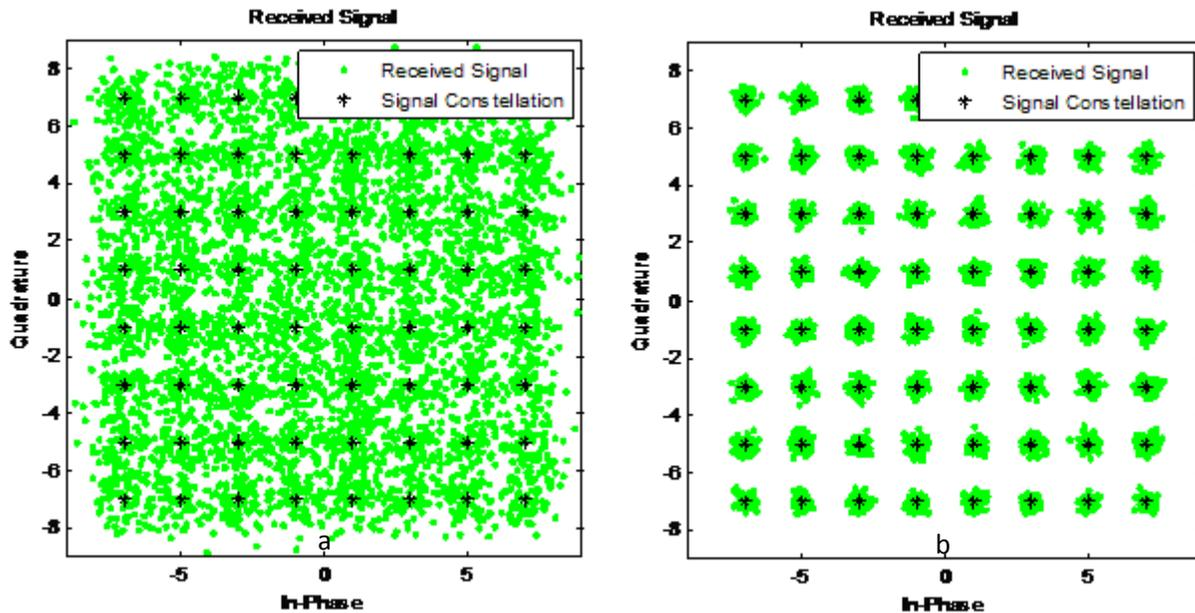
Figure 6 (a) and (b), constellation diagrams of the received 64-QAM signal, (a):  $E_b/N_0 = 10$  dB, (b):  $E_b/N_0 = 20$  dB.
