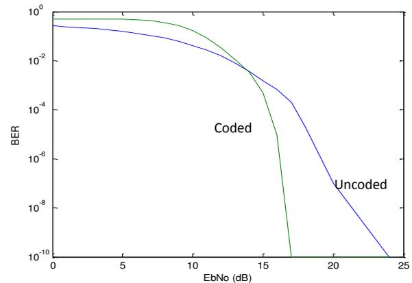
Figure 7, BER vs  $E_b/N_0$  for uncoded and convolutional coded 64-QAM signal
