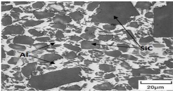
Figure1. 1 Al and sic particle in Metal Matrix [1]
