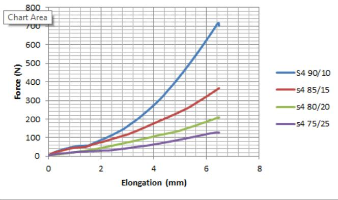
**Fig. 5. 2 Comparison among Force- elongation curves for various compositions of 4mm short fiber bio composites during tension**
