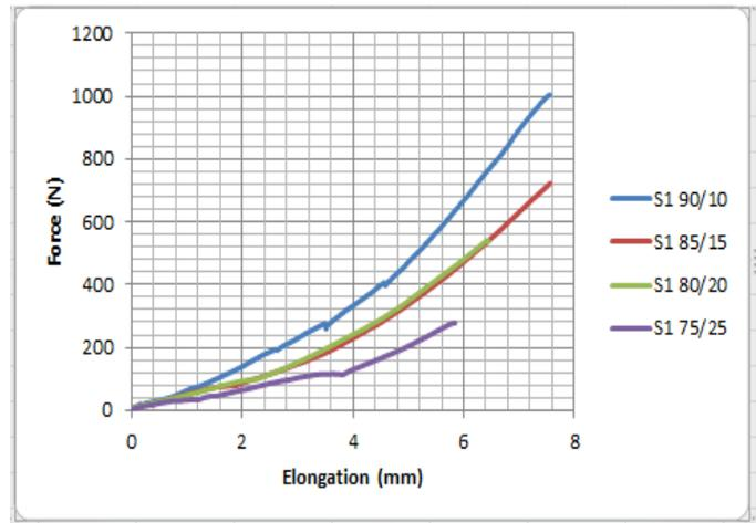
Fig. 5. 1 Comparison among Force- elongation curves for various composition of 1mm short fiber bio composites during tension
