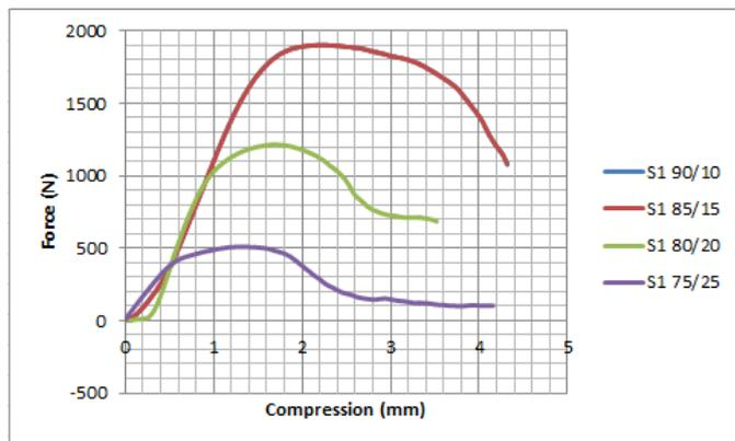
**Fig. 5. 3 Comparison among Force- elongation curves for various compositions of 1 mm short fiber bio composites during compression.**
