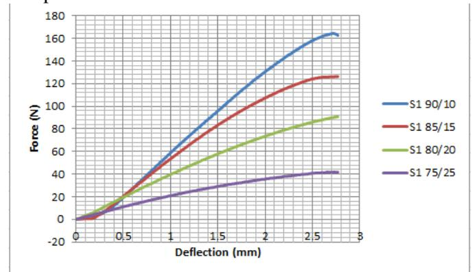
**Fig. 5. 7 Comparison among Force- elongation curves for various compositions of 1 mm short fiber bio composites during bending**
