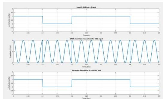
Figure 3: BPSK modulation and Demodulation
