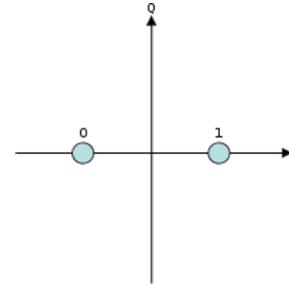
Figure 2: Constellation diagram for BPSK
