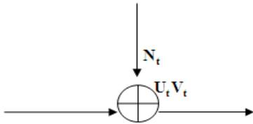
Figure 4: Blok diagram of AWGN classic
