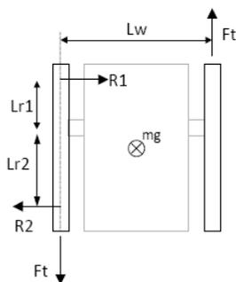
Fig -2: Static Load Case
