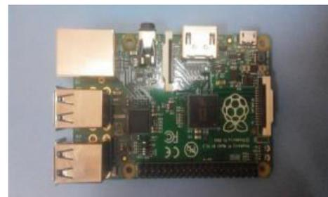
Fig.3 raspberry pi3 model B.
