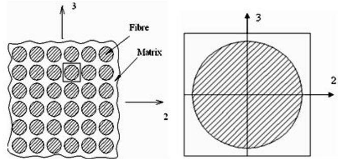
Fig: - 4 Concept of Unit Cells Isolated unit cells of square packed array
