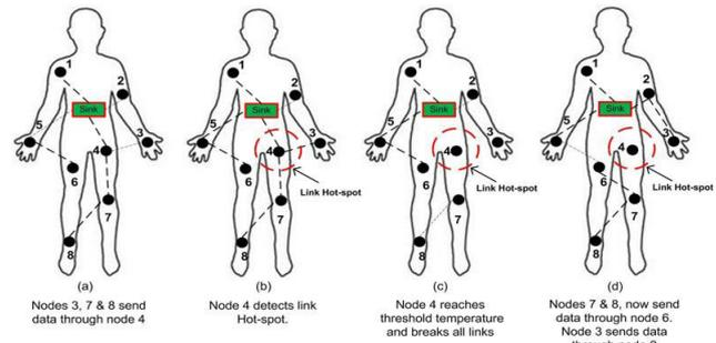
Fig 2: Link Hot-spot Detection
