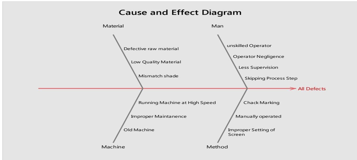
Fig 4: Cause and effect diagram.
