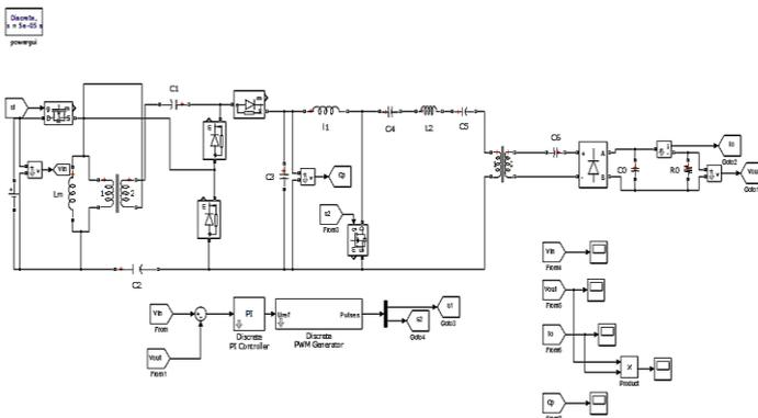
Figure 9, Circuit arrangement of the proposed wireless power transmission system using MATLAB/SIMULINK package.
