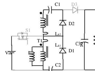
Figure 6, Mode IV operation of high step-up dc-dc converter
