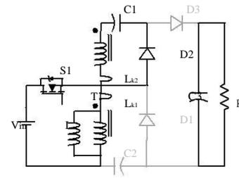
Figure 3, Mode I operation of high step-up dc-dc converter
