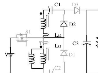
Figure 7, Mode V operation of high step up dc dc converter
