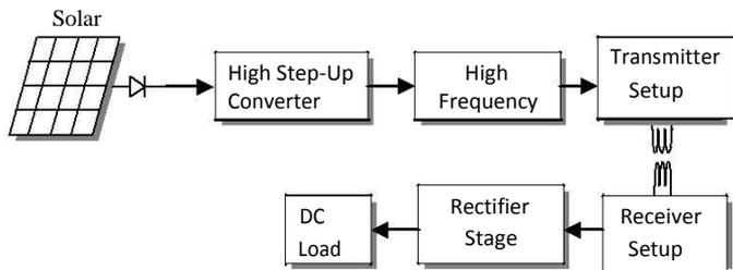
Fig 1, Block diagram of the proposed wireless power transmission system
