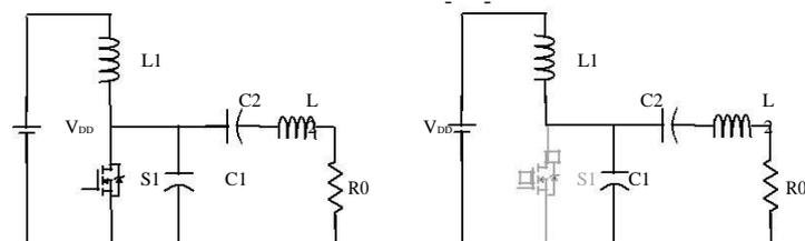
Figure 8, Operation of Class E Power Amplifier
