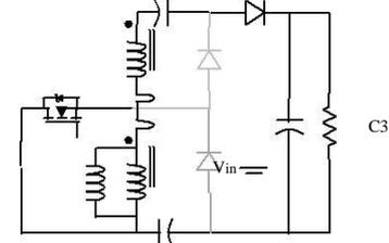
Figure 4, Mode II operation of high step-up dc-dc converter
