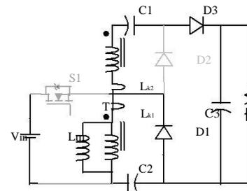
Figure 5, Mode III operation of high step-up dc-dc converter
