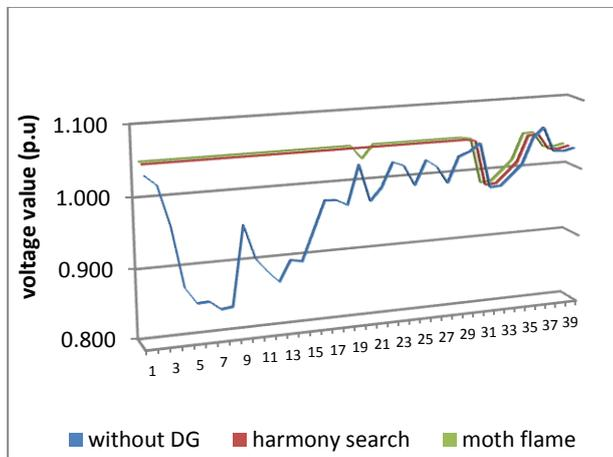
Fig (10) Voltage Profile of IEEE-39 Bus System with Hydro Power DGs
