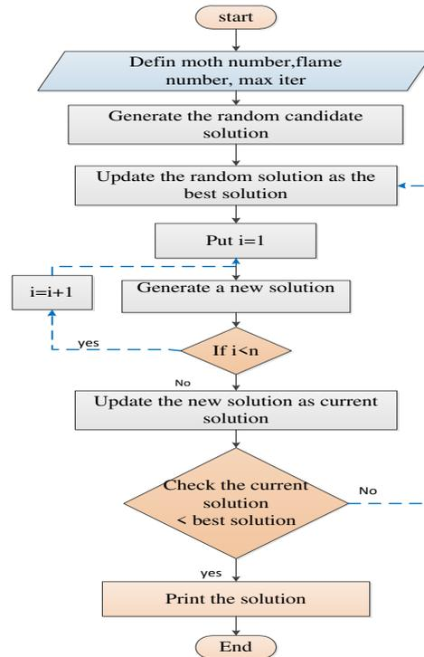
Fig (3) Flowchart of Moth Flame Optimization Technique
