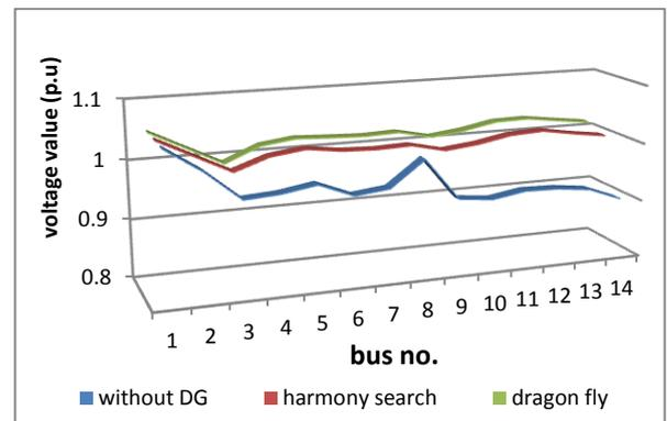
Fig (5) Voltage Profile of IEEE-14 Bus System for windTurbine DGs Technology
