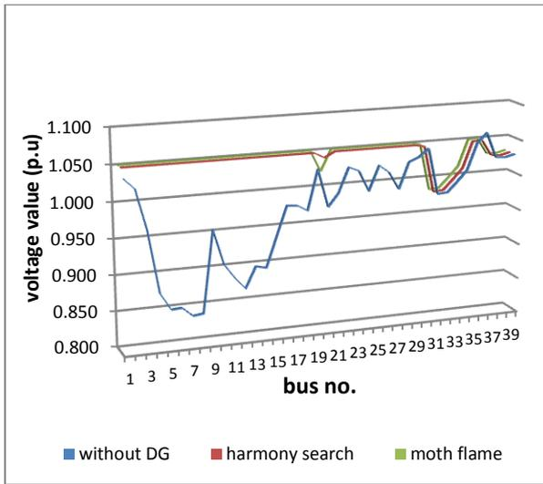
Fig(9) Voltage Profile of IEEE-39 Bus System with Combined cycle DGs
