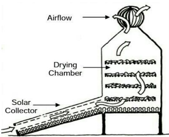
**Figure 4:** Working principle of an Indirect Solar Drying (ISD) Source; Sharma et al 2009
