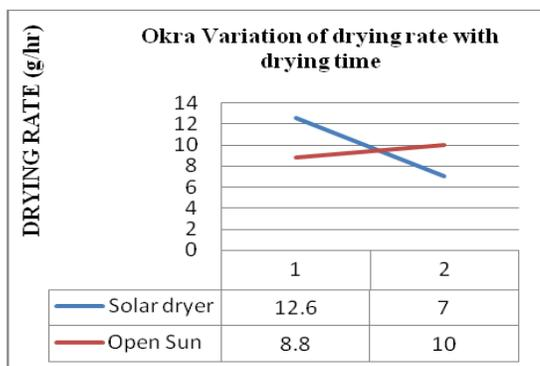
**Figure 7;** Variation of Drying Rate with drying time (hour) of okra using solar dryer and open sun. Source; from table above.
