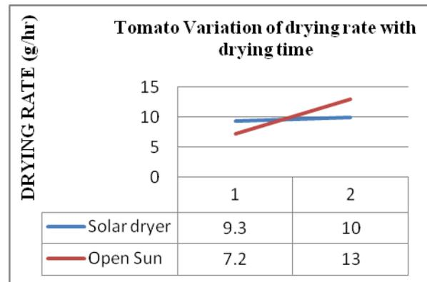
**Figure 8;**Variation of Drying Rate with drying time (h) of Tomato using solar dryer and open sun. Source; from table 4 above
