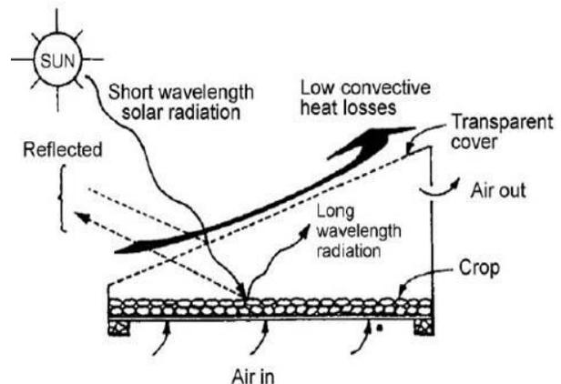
**Figure 5:** Working principle of direct solar drying.
