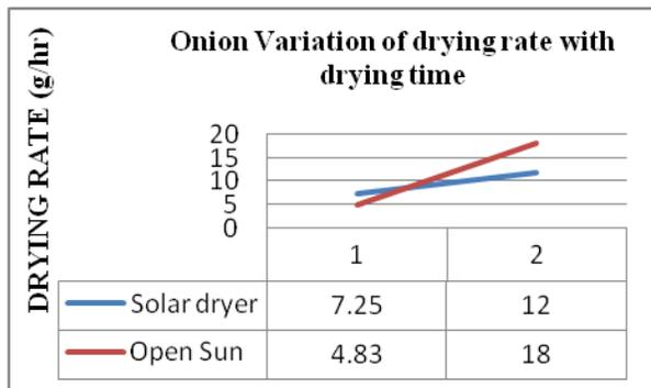
**Figure 6;** Variation of Drying Rate with drying time (hour) of onion using solar dryer and open sun. Source; from table 4 above
