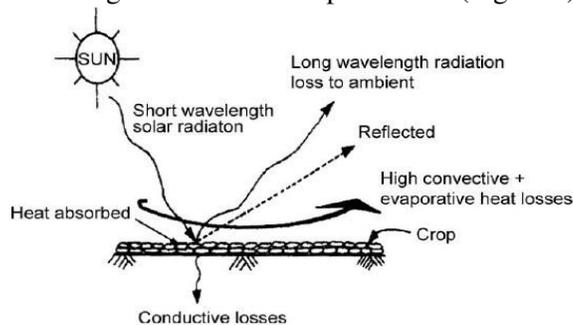
**Figure 2:** Working principle of Open sun drying
