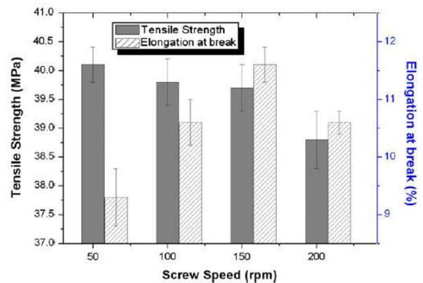
Figure 3: Tensile strength and elongation at break for different extruder screw speed [21].
