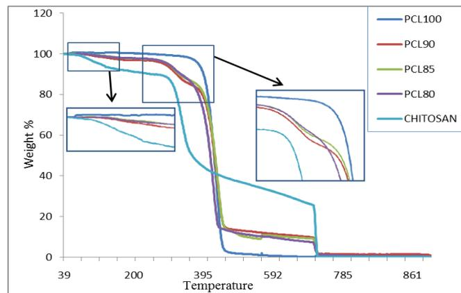
Fig. 1 TGA curves for PCL and PCL-Chitosan with various compositions
