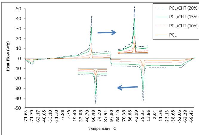
Fig. 2 DSC thermograms for PCL and PCL-CHT biocomposites with various CHT content during heating time.
