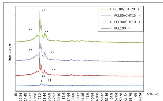
Fig. 4 Pattern of XRD of PCL-CHT composite with different wt%. of chitosan loading (0, 10, 15, and 20).
