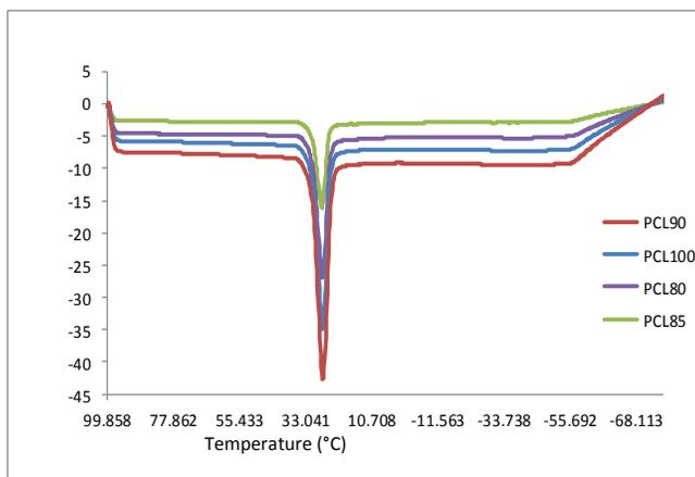
Fig. 3 DSC thermograms for PCL and PCL-CHT biocomposites with various CHT content during cooling time.
