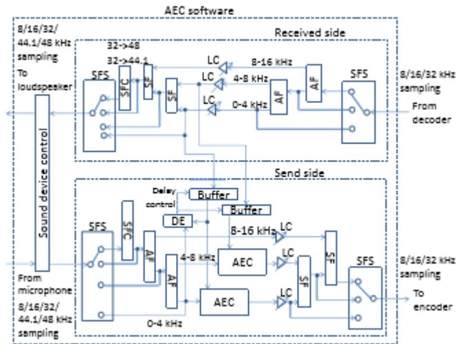
**Fig.2 Block diagram of AEC software implemented in VOIP application.**
