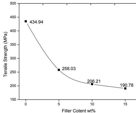
**Fig. 3. Tensile strength vs filler content**
