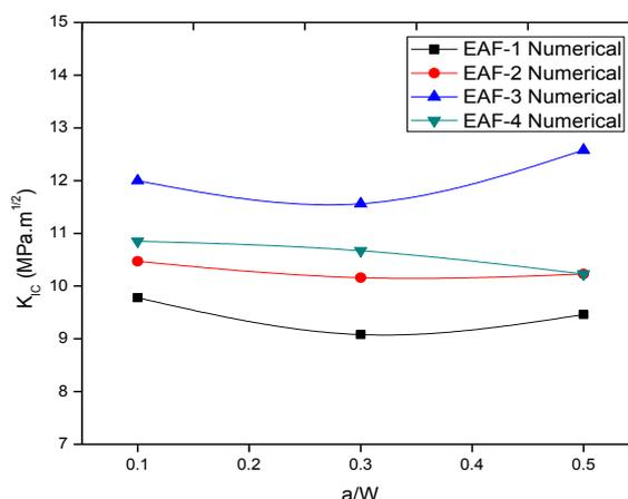
**Fig. 8. Variation of numerical stress intensity factor of marble dust filled aramid epoxy composites.**
