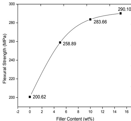
**Fig. 5. Flexural strength vs filler content**
