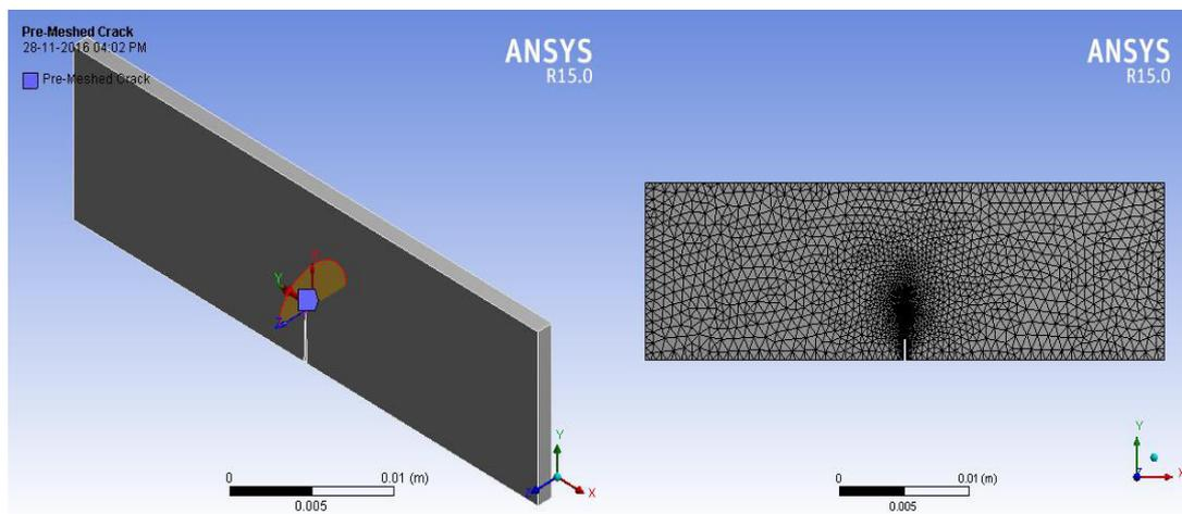
**Fig. 1. Pre-meshed crack and type of mesh generated**
