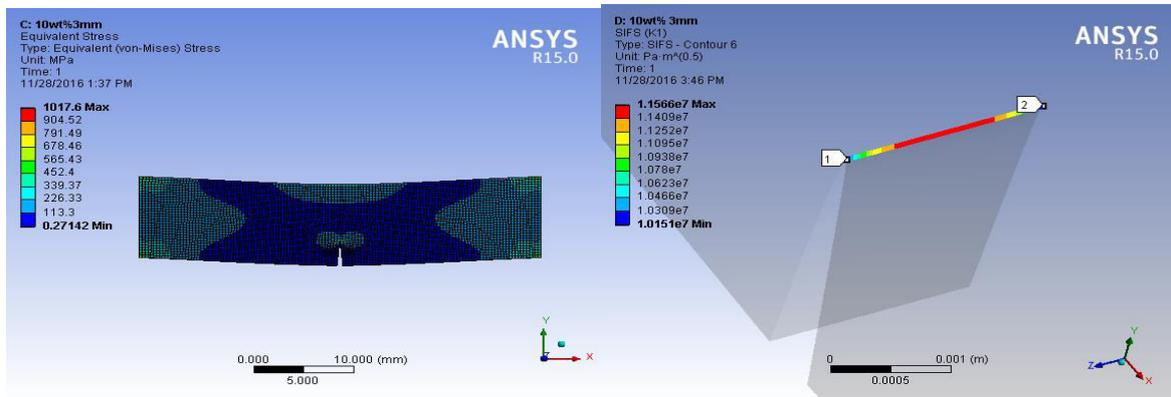
**Fig. 9.(a) and(b) shows the equivalent von-misses stress contour and stress intensity factor ( $K_{IC}$ ) with  $a/W$  ratio as 0.5 along the crack front**
