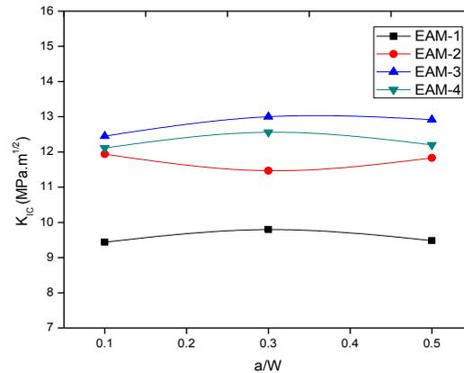
**Fig. 7. Variation of stress intensity factor of marble dust filled aramid fibre reinforced epoxy composites**
