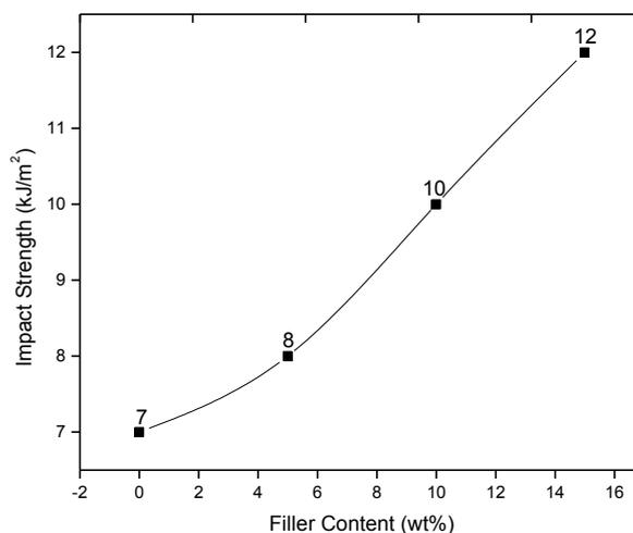
**Fig. 6. Impact strength vs filler content**
