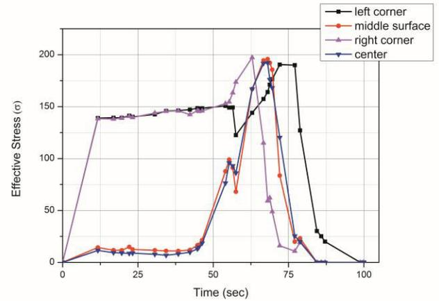
Fig. 8 Effective stress of square case versus time
