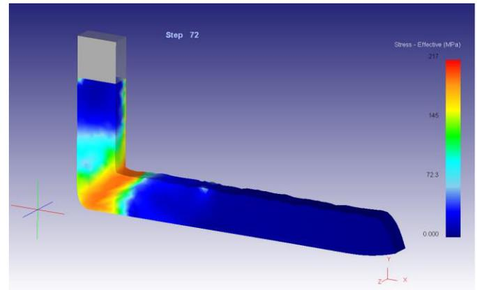
Fig. 4 Effective stress distribution from vertical symmetry surface while pressing
