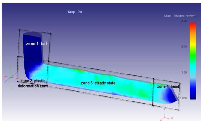
Fig. 3 ECAP zones and effective strain distribution
