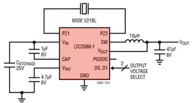
Fig. 2 Piezoelectric energy harvesting power supply
