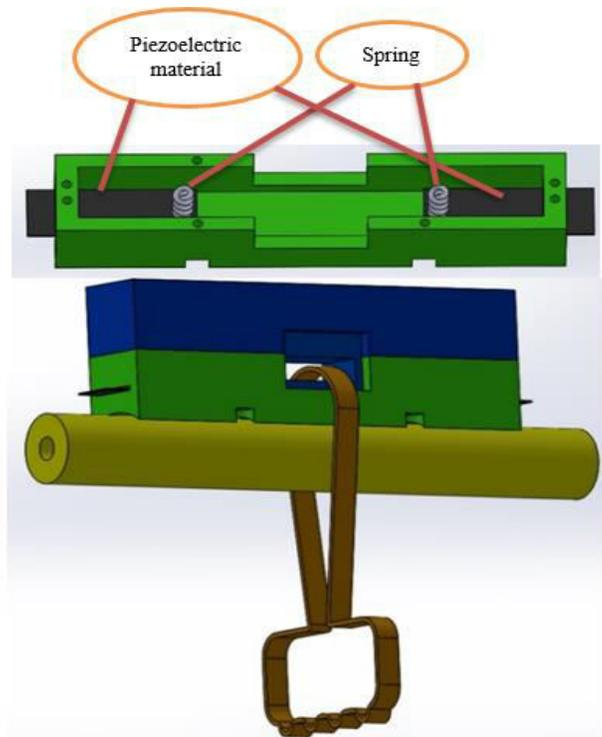
Fig. 1 Prototype hand holder system solid model
