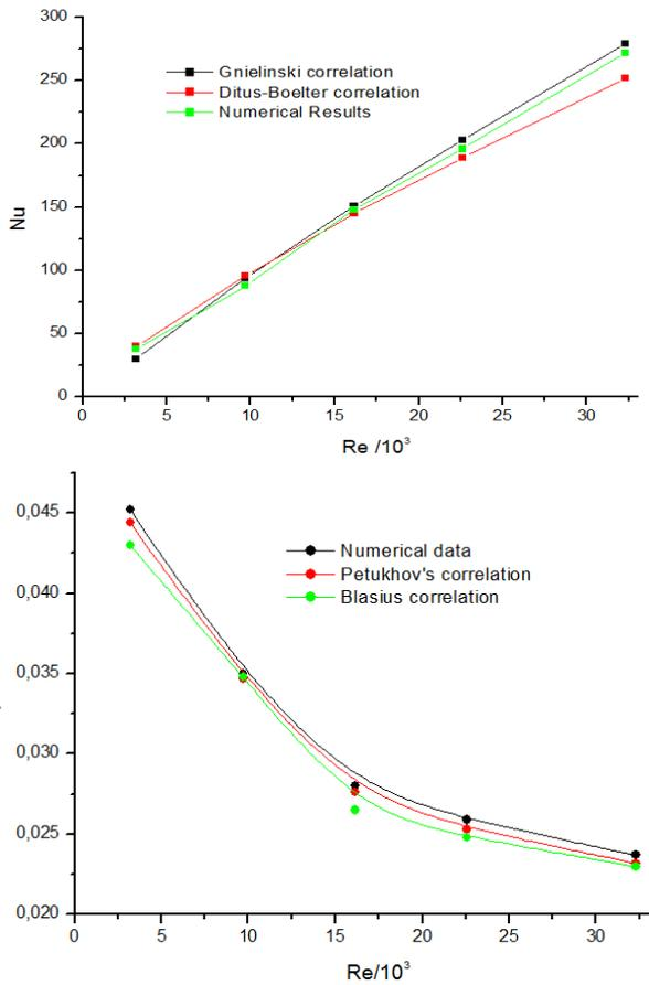
Fig. 4: Validation of numerical results for a smooth absorber.
