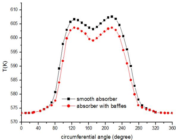
**Fig.8:** absorber temperature distribution on the middle cross-section.
