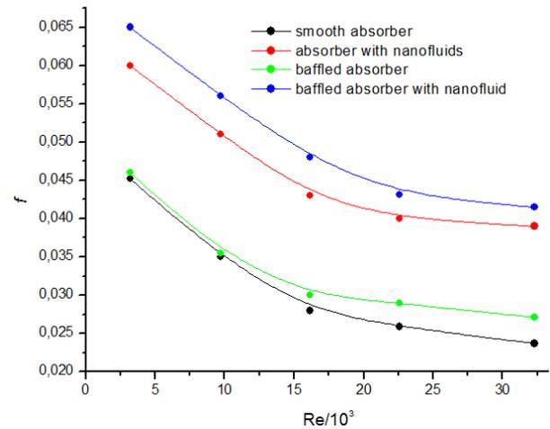
Fig.14: effect of baffles and nanofluid on pressure drop
