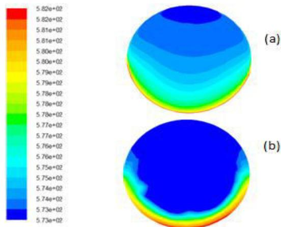
Fig.7: HTF Temperature distribution for smooth tube (a) and baffled tube (b).
