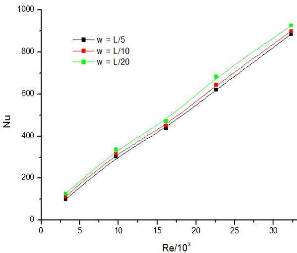
Fig.11: Effect of distance between two consecutive baffles on heat transfer.
