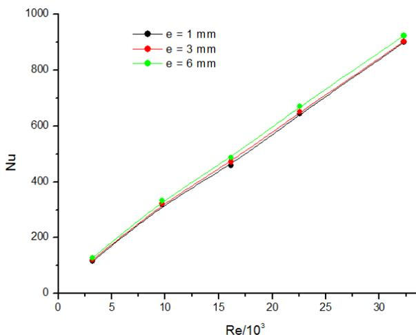
Fig.12: Effect of baffles thickness on Nusselt number.
