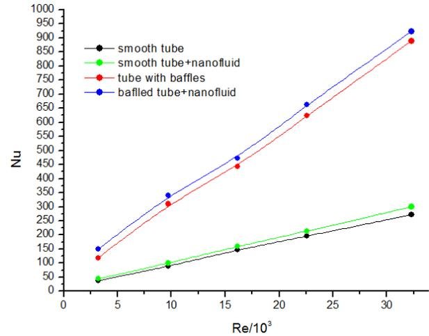
Fig.13 Effect of using baffles and nanofluid on heat transfer characteristics
