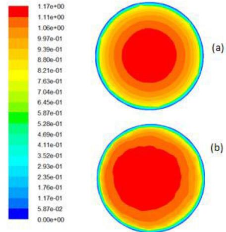
**Fig. 10:** HTF Velocity distributions on the middle cross-section.
