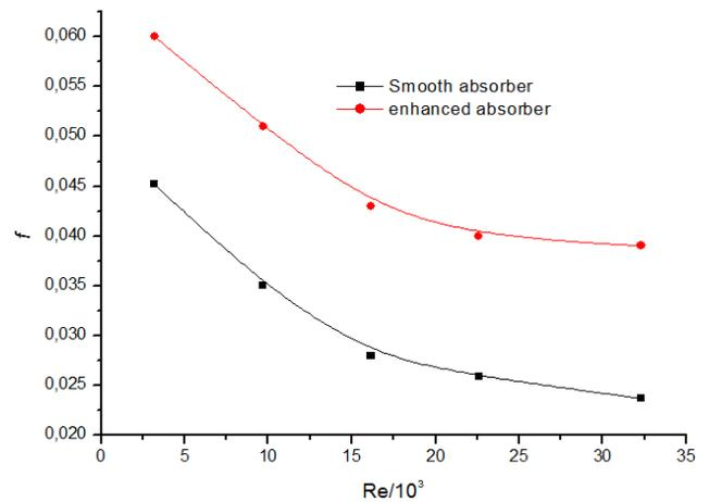
Fig.6: Evolution of friction factor for tube with and without baffles.
