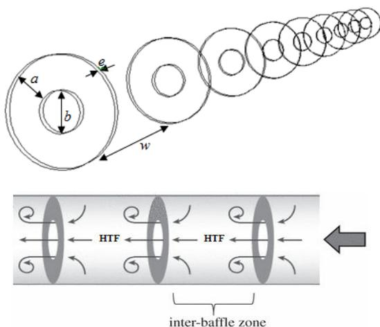
Fig. 2: Model configuration with geometrical parameters.
