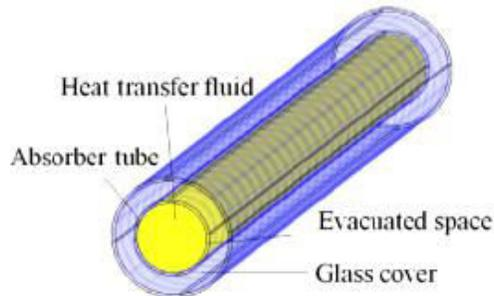
Fig. 1: schematic of PTC receiver
