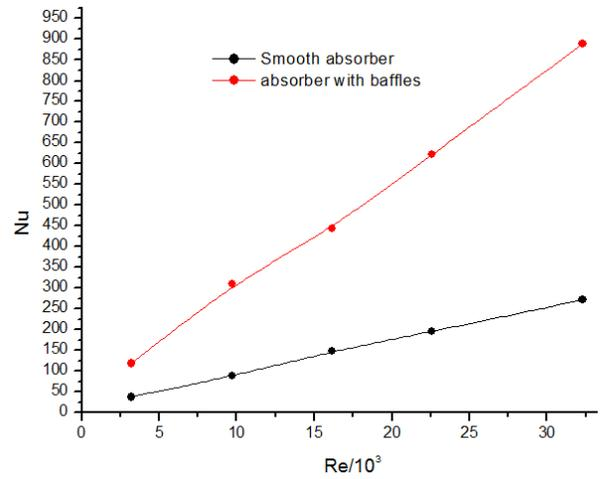
Fig.5: Variation of Nusselt number for tube with and without baffles.
