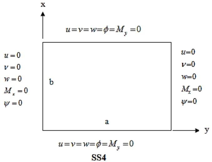
**Fig. (1) Simply supported boundary conditions**
