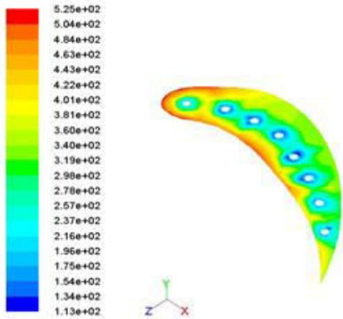
Fig.16 Variation of static temperature of 8 holes
