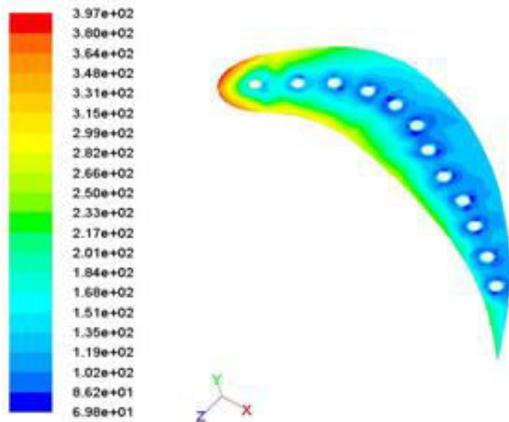
Fig.18 Variation of static temperature of 12 Holes Nickel alloy in Gas Turbine Blade.
