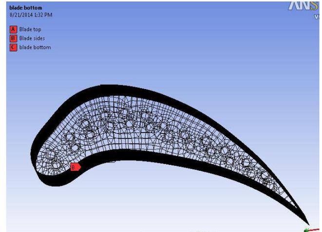
Fig.8 Meshing of 12 holes gas turbine blade
