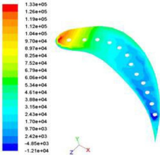
Fig.17 Variation of static pressure of 12 holes Nickel alloy in Gas Turbine Blade.
