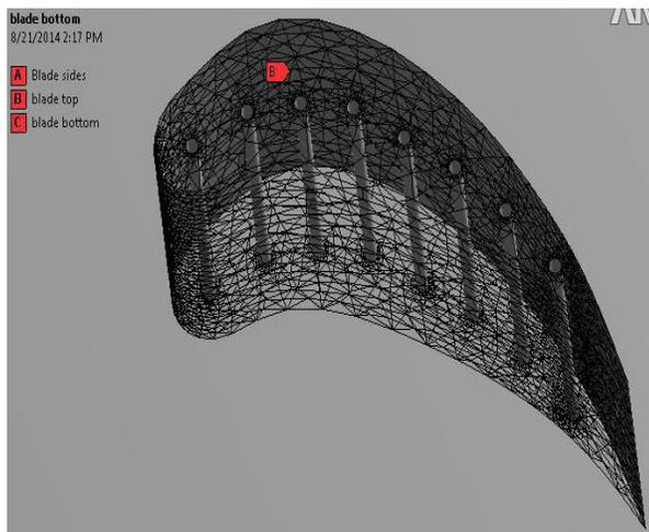
Fig. 7 Meshing of 8 holes gas turbine blade
