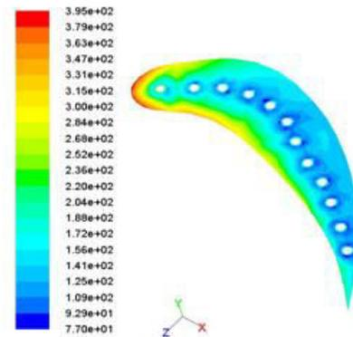
Fig.20 Variation of static temperature of 12 holes
