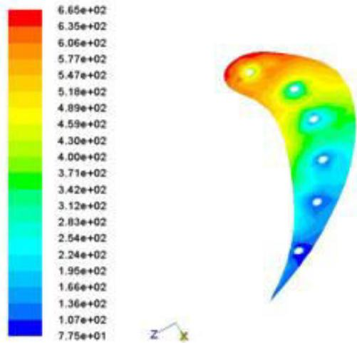
Fig. 10 Variation of static temperature of 6 Holes Nickel alloy in Gas Turbine blade.
