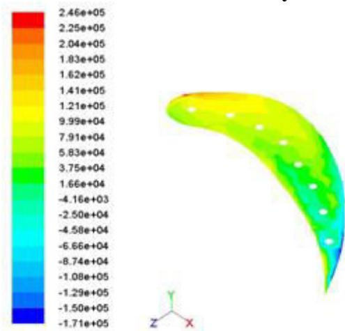
Fig. 15 Variation of static pressure of 8 holes Titanium alloy in Gas Turbine Blade.
