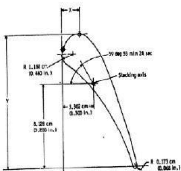
Fig.2 Schematic of the gas turbine blade
