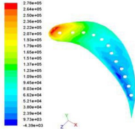
Fig.19 Variation of static pressure of 12 holes Titanium alloy in Gas Turbine Blade.
