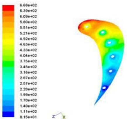
Fig. 12 Variation of static Temperature of 6 Holes
