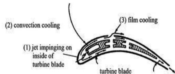
Fig.1 Types of cooling methods
