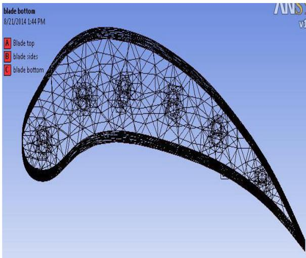
Fig. 6 Meshing of 6 holes gas turbine blade
