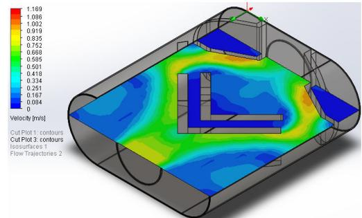
Fig. 10 Cut plot of Design-2 showing velocity
