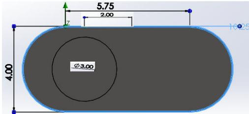
Fig.1 Front View of Design-1 with inlet position
