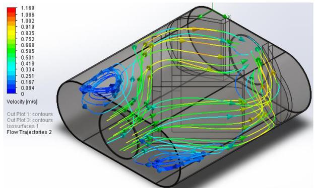
Fig. 11 Flow trajectories with velocity as parameter
