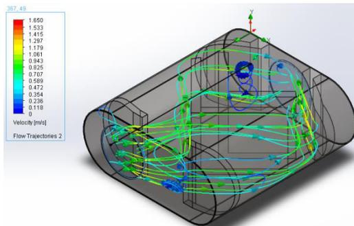
Fig. 7 Flow trajectories with velocity as parameter in Design-1
