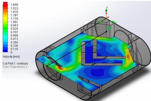
Fig. 6 Cut plot of Design-1 showing velocity distribution
