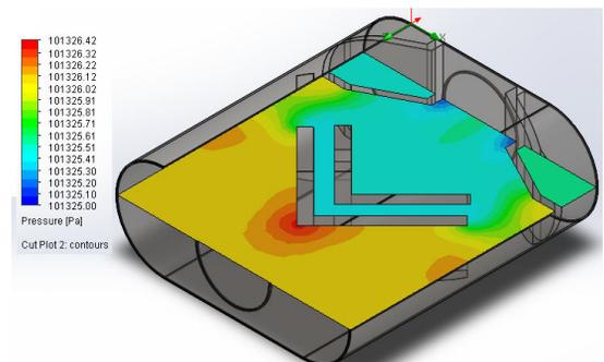
Fig. 12. Cut plot of Design-2 showing pressure distribution
