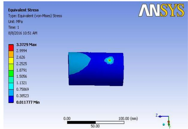
**Fig 4: Drill jig component (Mandrel) – Equivalent Stress**
