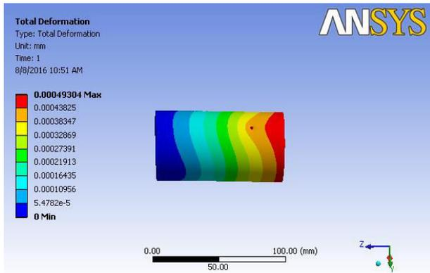
Fig.5 Drill jig component (Mandrel) –Total Deformation
