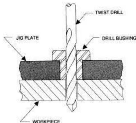
**Fig 1:** A Jig guides the cutting tool, in this case with a bushing
