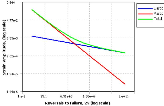
Structural Steel > Strain-Life Parameters > Strain-Life Parameters
