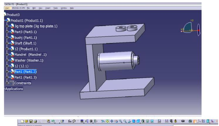
Fig 2: CATIA V5R20 Model of Assembled Drill Jig
