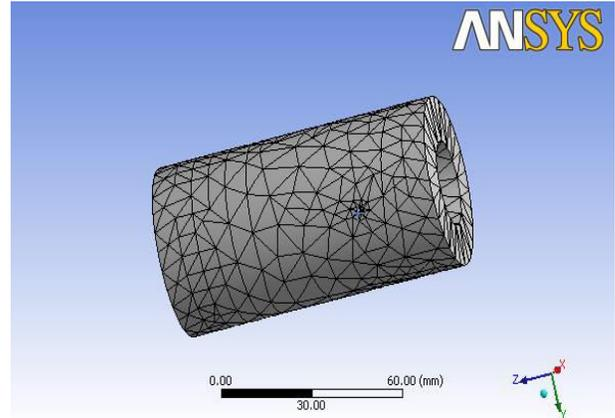
**Fig 3: Drill jig component (Mandrel) - Meshed**
