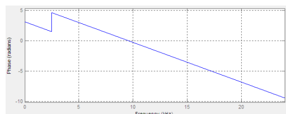
Figure 2: Phase Response of Hamming Window Technique
