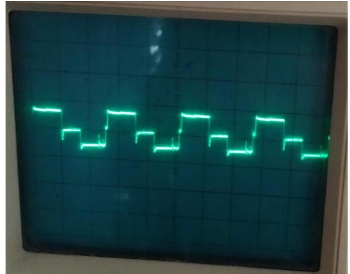
Fig 4: Three level inverter output across primary of transformer
