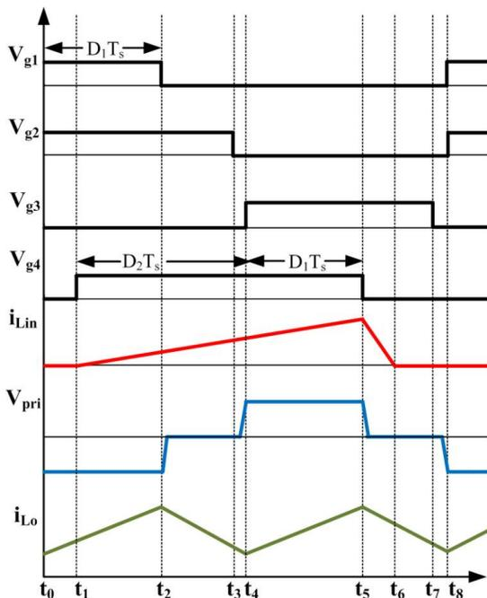
Fig 2: Typical waveforms of the converter
