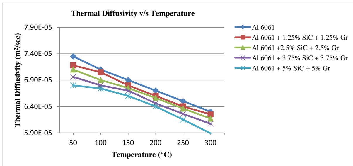
**Fig. 7. Variation of Thermal Diffusivity with Temperature for Varying Mass Fraction of MMCs**
