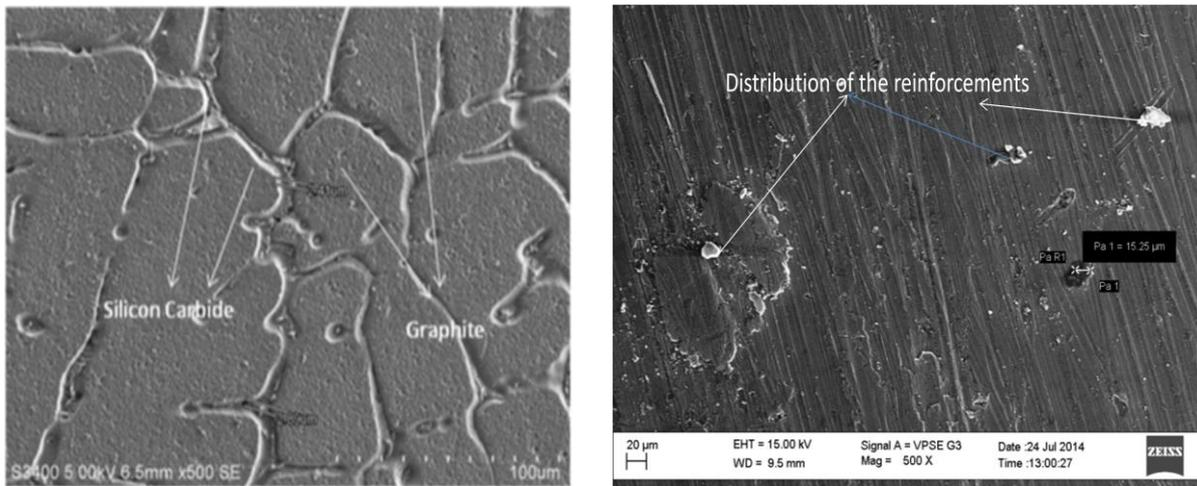
**Fig. 4 (a) and (b) Microstructures of Al 6061 with 3.75% Silicon Carbide and 3.75% Graphite**
