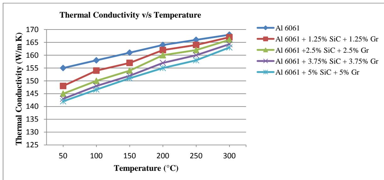
**Fig. 8. Variation of Thermal Conductivity with Temperature for different compositions of MMCs**
