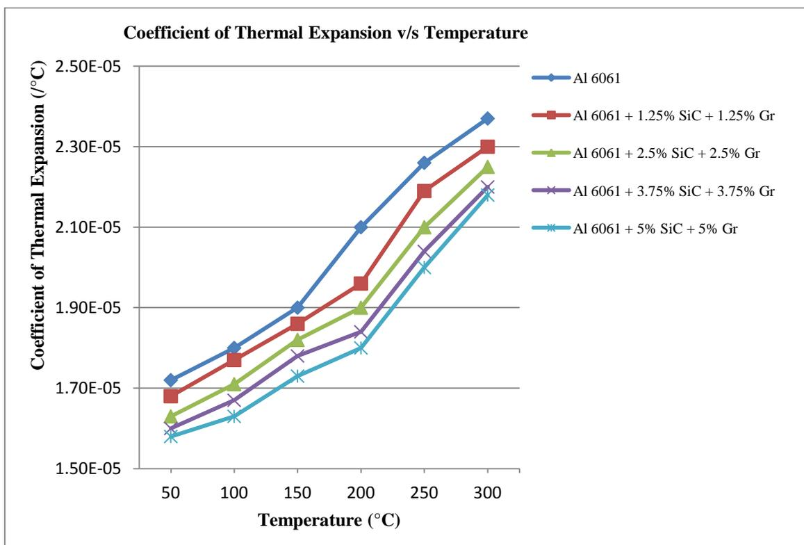
Fig. 9. Variation of CTE with Temperature of Hybrid Composites
