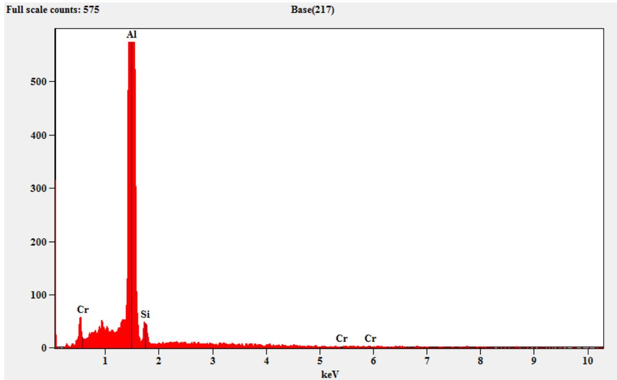
**Fig. 6. Elemental Compositions of Al 6061 + 2.5% SiC + 2.5% Gr**
