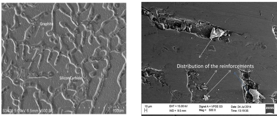
**Fig. 5 (a) and (b) Microstructures of Al 6061 with 5% Silicon Carbide and 5% Graphite**
