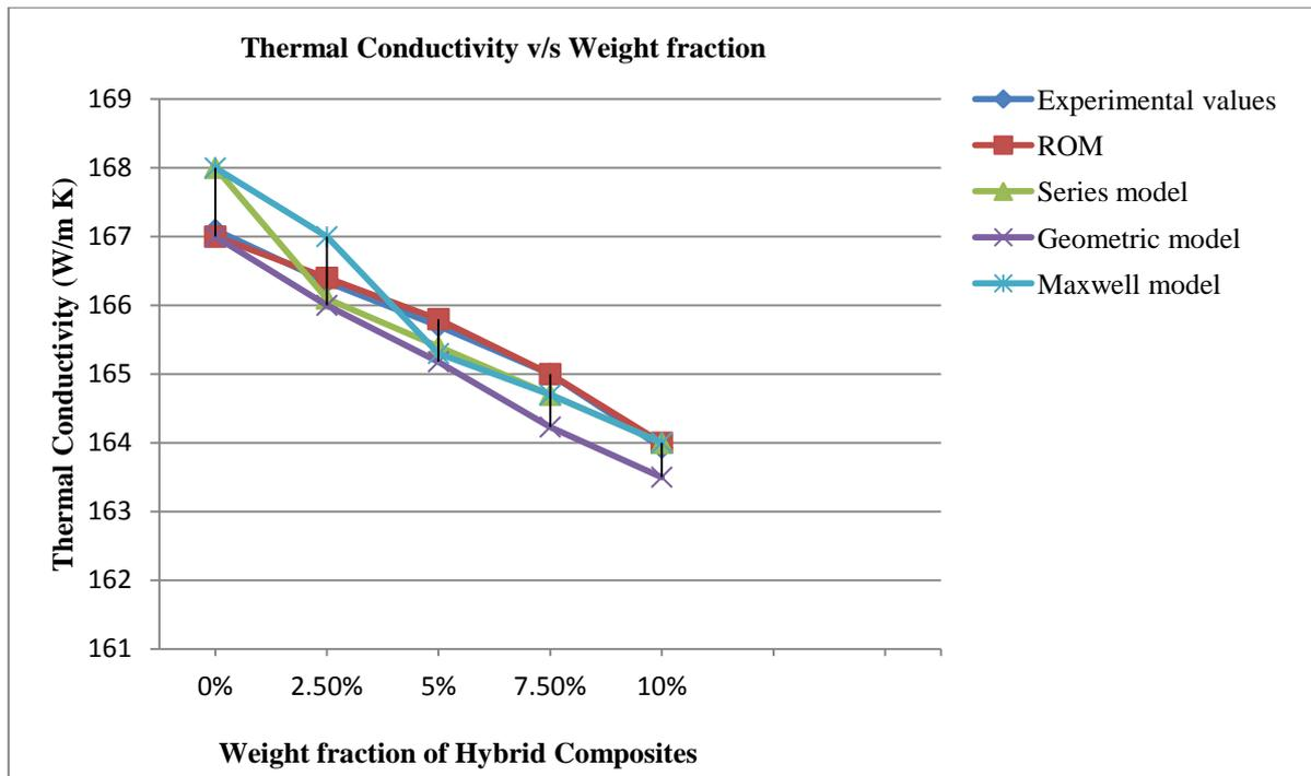
**Fig. 10. Validation of the Thermo-elastic Models with Experimental Results**
