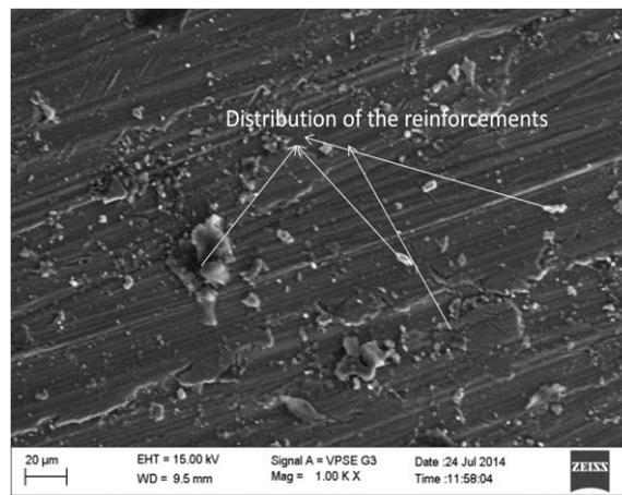
**Fig. 3 (a) and (b) Microstructures of Al 6061 with 2.5% Silicon Carbide and 2.5% Graphite**
