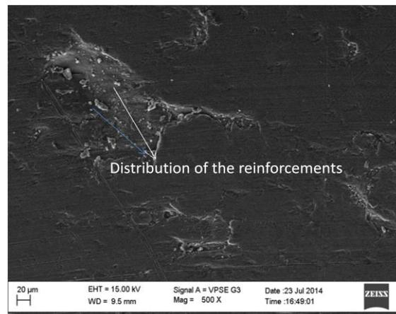
**Fig. 2 (a) and (b) Microstructures of Al 6061 with 1.25% Silicon Carbide and 1.25% Graphite**
