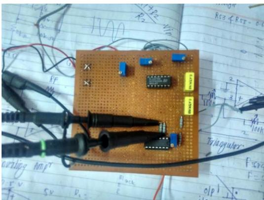
Fig 5 Integrator Circuit
