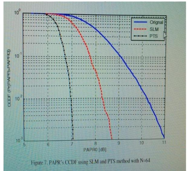
Figure 7. PAPR's CCDF using SLM and PTS method with N=64
