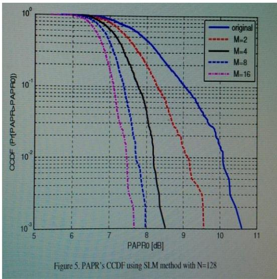
Figure 5. PAPR's CCDF using SLM method with N=128
