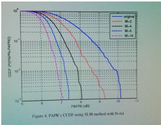
Figure 4. PAPR's CCDF using SLM method with N=64
