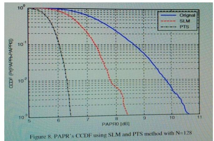
Figure 8. PAPR's CCDF using SLM and PTS method with N=128
