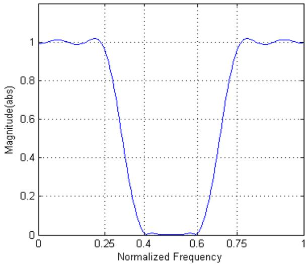
Fig. 3 Magnitude (abs) plot for the FIR BS filter Order 22
