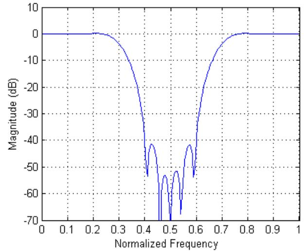
Fig. 2 Magnitude (dB) plot for the FIR BS Filter of order 22
