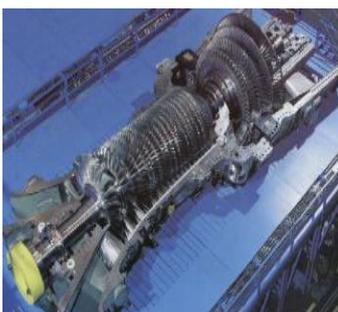
Fig 1. Gas Turbine Simple Open Cycle
