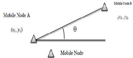
Fig. 3: Position-based routing protocol that uses GPS to determine mobile nodes (x, y) positions.
